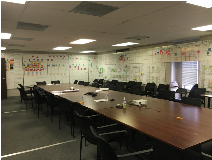
Figure 1: Last Planner System "In Action" Source: Clark Construction; Los Angeles U.S. Courthouse Project Date Taken: April 22, 2016
