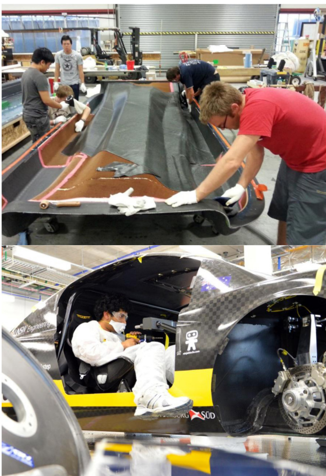
Figure 10. Experience not available in the classroom: the composites team travelled to New Zealand in 2013 to fabricate the moulds and car shells for eVe with industry partner Core Builders Composites (top), then completed the manufacture and assembly of the entire vehicle at UNSW in approximately 4 months (bottom).
