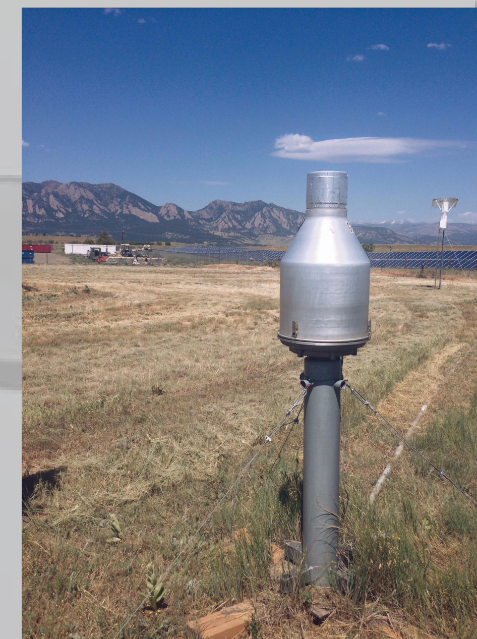
Fig. 2 (above) A GEONOR T-200B All-Weather Precipitation Gauge can be used to measure the liquid water equivalences if frozen precipitation falling at airports.
