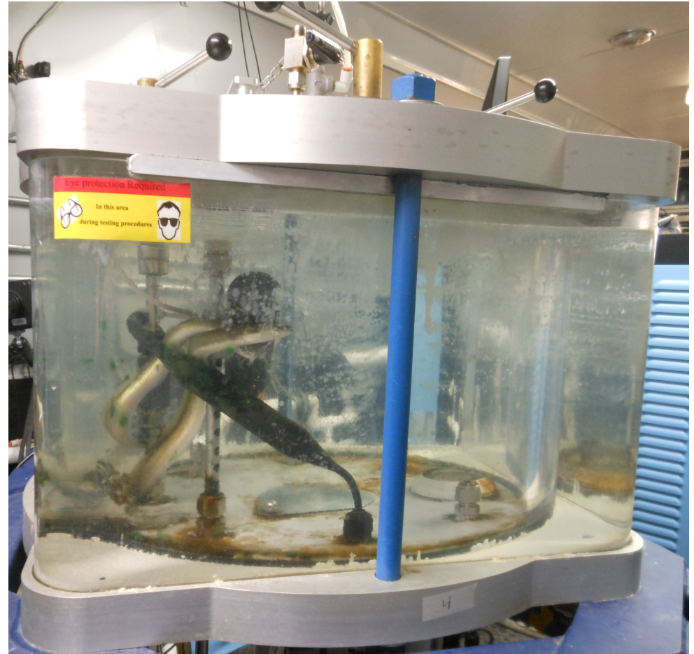
Eels in chamber being acclimated to 25 psi (equivalent of 25 ft depth)
