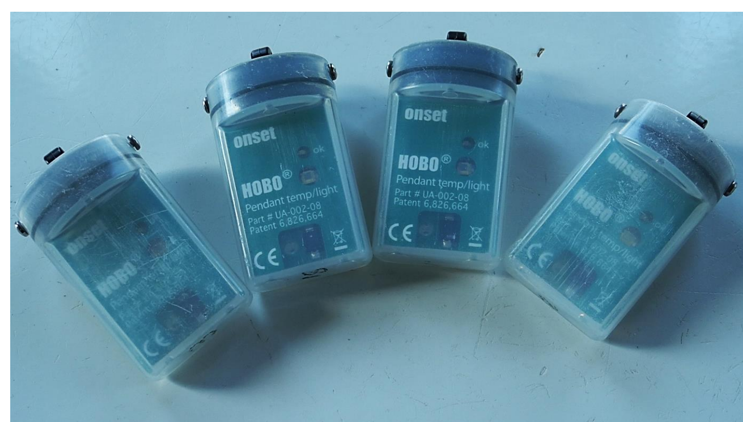
Figure 3: HOBO pendant light and temperature sensors.
