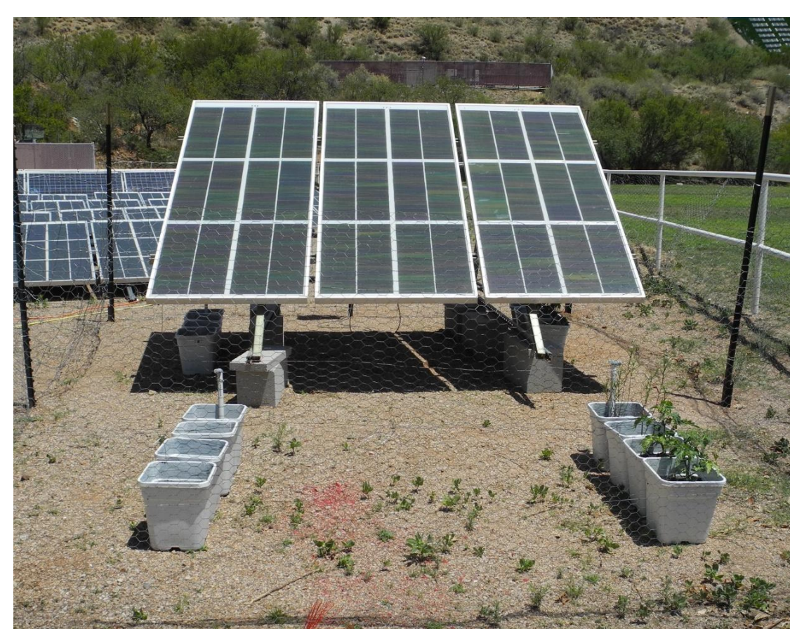
Figure 2: Experimental set-up. Photo is taken facing north. Shaded plants are on the right side of the photo underneath the panel; shaded soil is on the left. Unshaded plants and soil are in the foreground.
