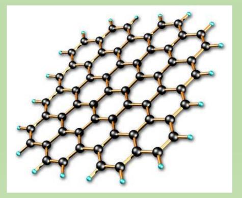
Figure 2. Graphene's 2-D structure. A single layer is only an atom thick.
