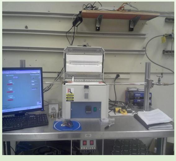
Figure 3. Furnace used for CVD
