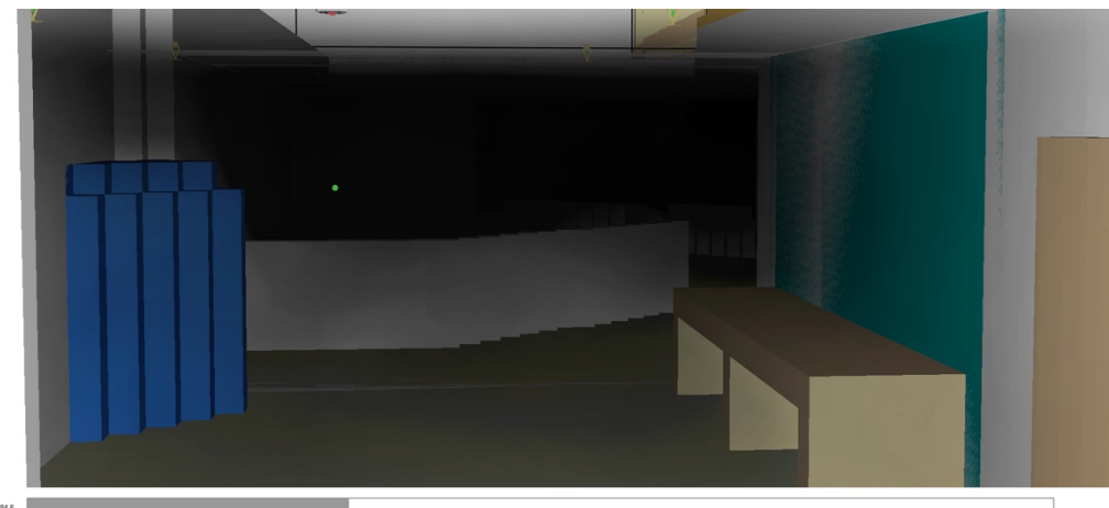
Figure #96: Lobby Fire – Smoke only – 2 nd Floor looking south from dead end hallway (87.6s) Visibility tenability failed in second floor lobby (15 seconds after detection)
