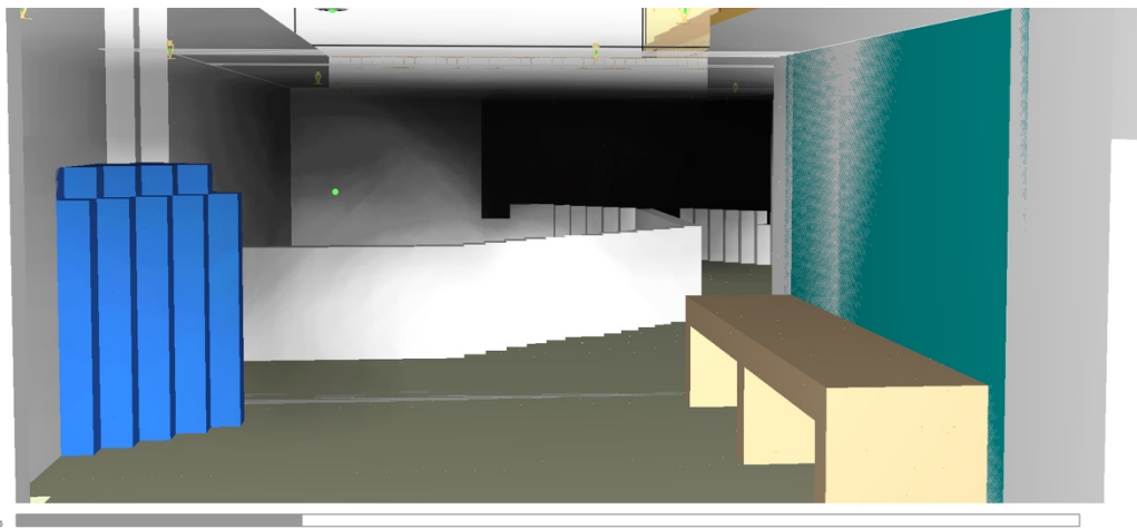
Figure #95: Lobby Fire – Smoke only – 2 nd Floor looking south from dead end hallway (72.6s) Activation of the smoke detector directly above this location
