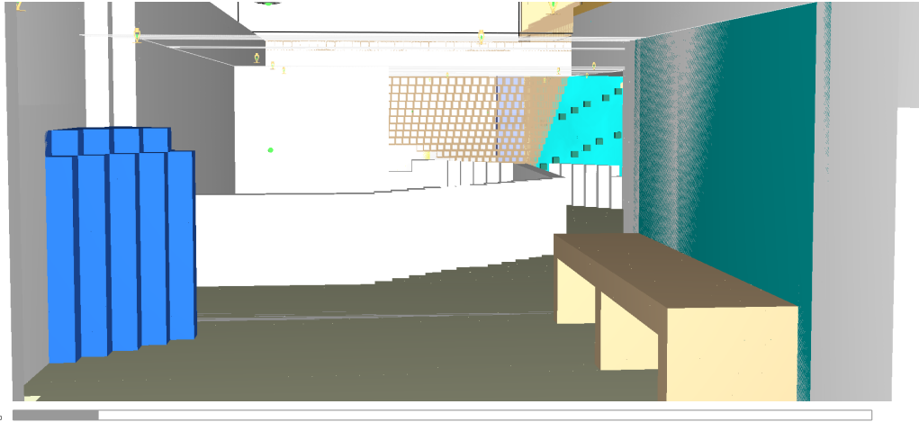
Figure #94: Lobby Fire – Smoke only – 2 nd Floor looking south from dead end hallway (27.0s) Visible fire detection in the lobby
