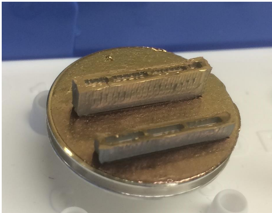
Figure 15: Gold coating applied to the cross section of the sample.
