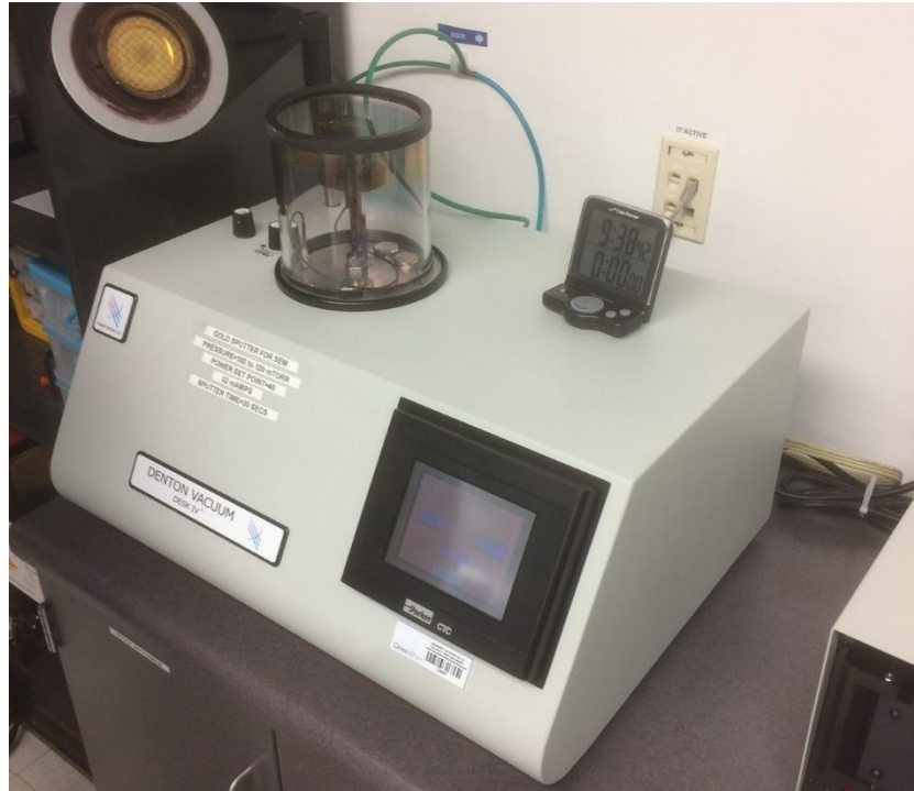
Figure 12: Sputtering Machine used to deposit gold on the surface of the print. This is done so that the SEM can be used in this experiment.
