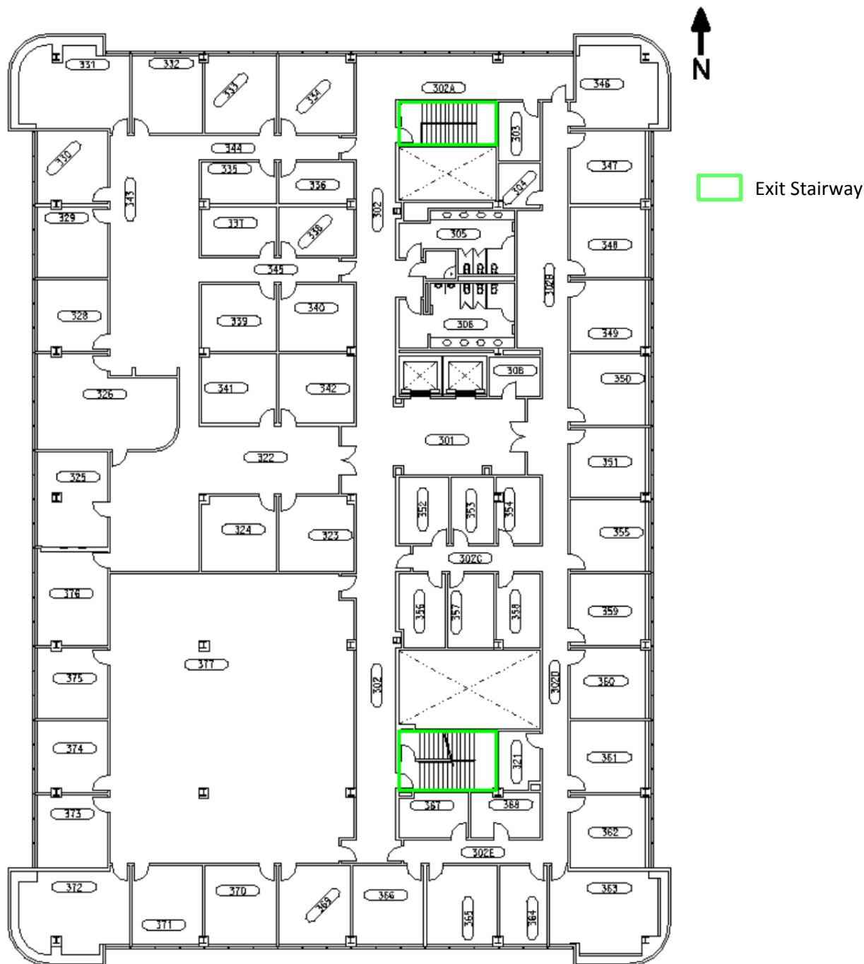
Figure 17: Exit Layout - Third Floor
