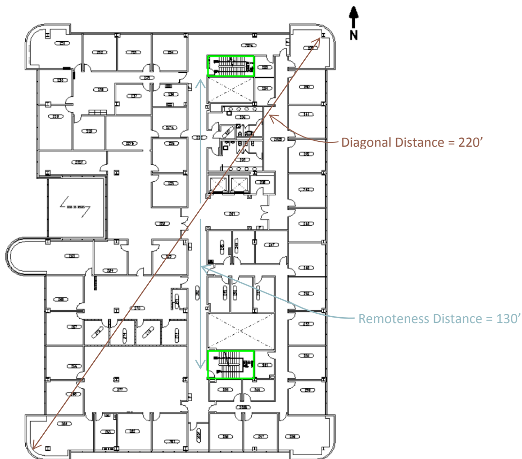
Figure 13: Exit Stairway Remoteness Layout (Second Floor)
