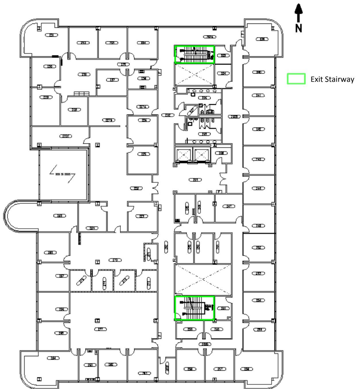
Figure 16: Exit Layout - Second Floor
