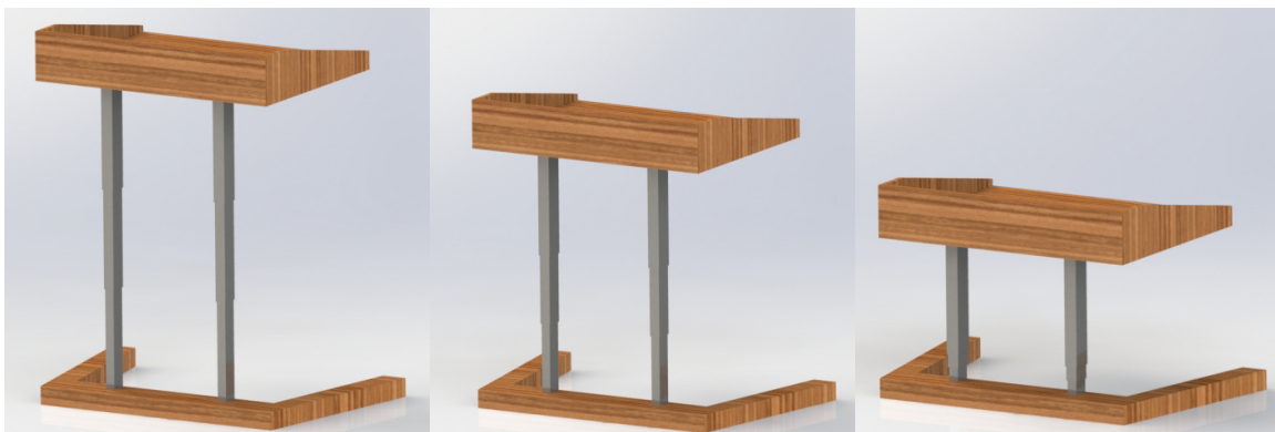
Figure 10. 3-D model of off-the-shelf system at various height positions
