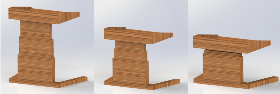
Figure 11. Motion of privacy panels through adjustment range
