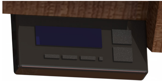
Figure 48. CAD model of Workrite height adjustment control module
