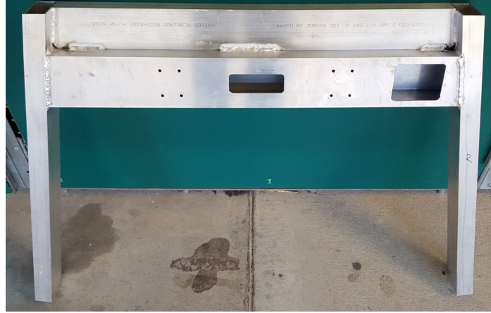
Figure 62. Fully Welded Aluminum Subframe
