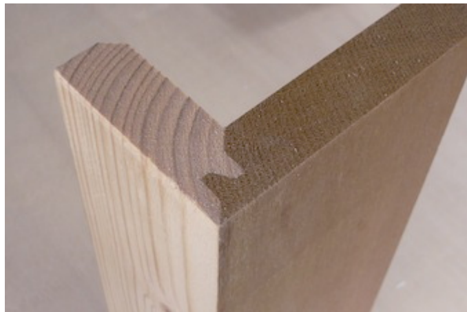
Figure 38. Lock miter joint
