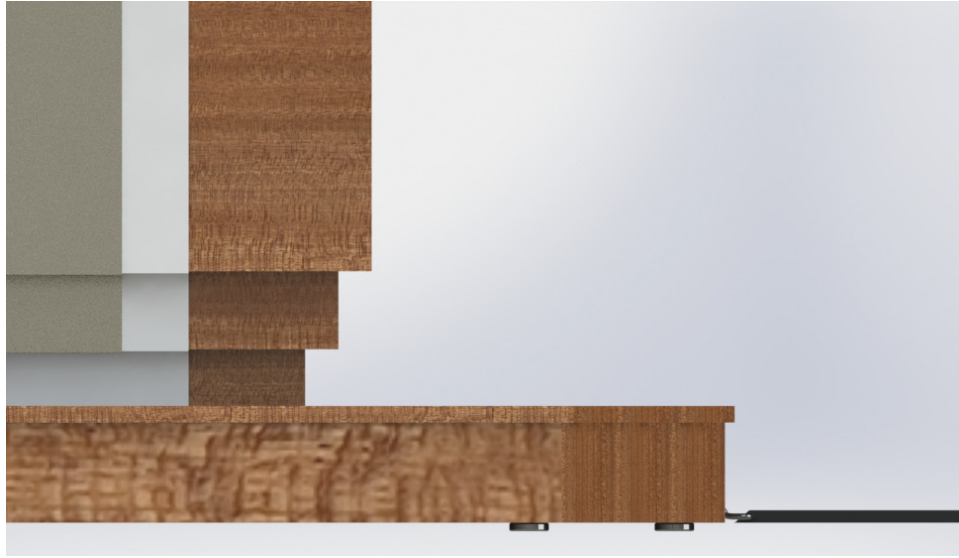
Figure 32. Feet and frame clearance
