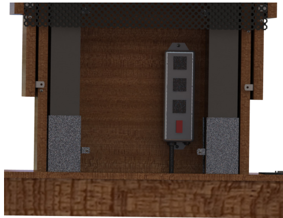
Figure 54. Power strip mounting location
