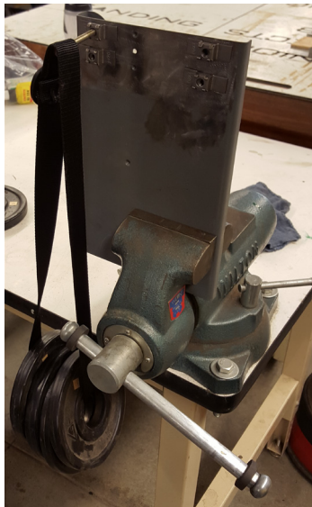
Figure 81. Weld nut test configuration with ten pound load
