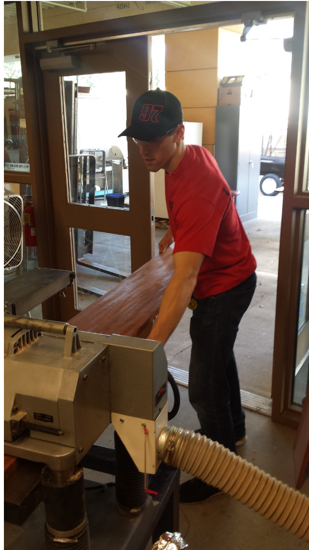
Figure 63. Planing boards to 1/2" for sides of base
