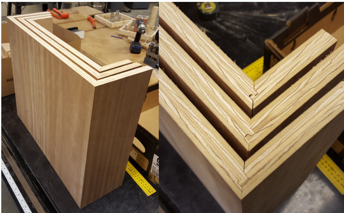
Figure 67. Cascading covers and close-up of lock miter joints
