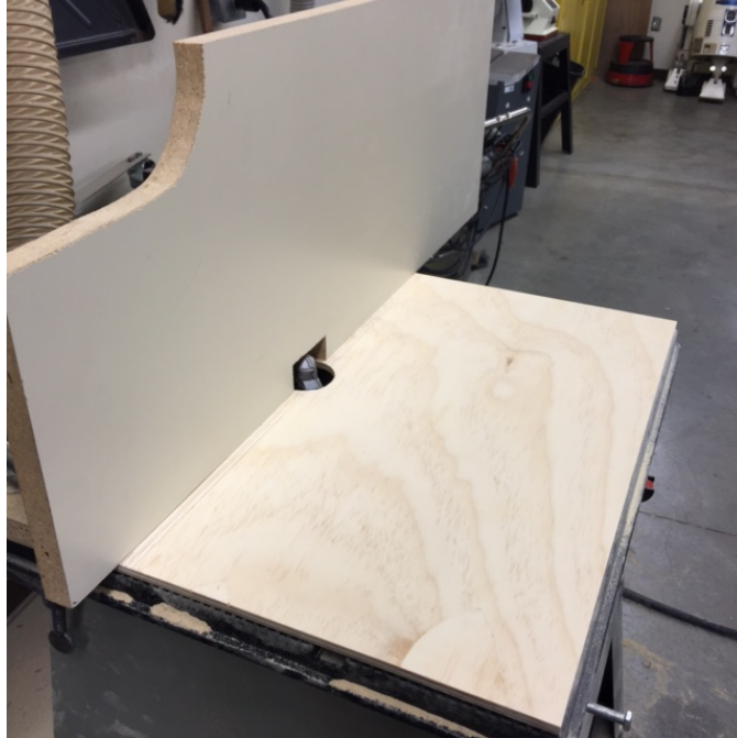
Figure 66. Router table setup for cutting of lock miter joint
