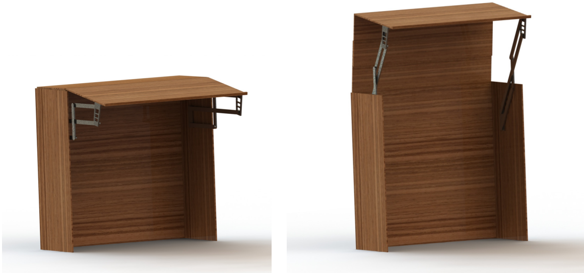
Figure 17. Mechanical linkage solution in fully collapsed and fully extended positions
