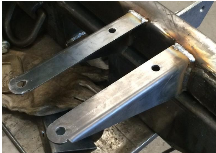
Figure 29. Jerry (fuel) can mounting bracket installed on rack.
