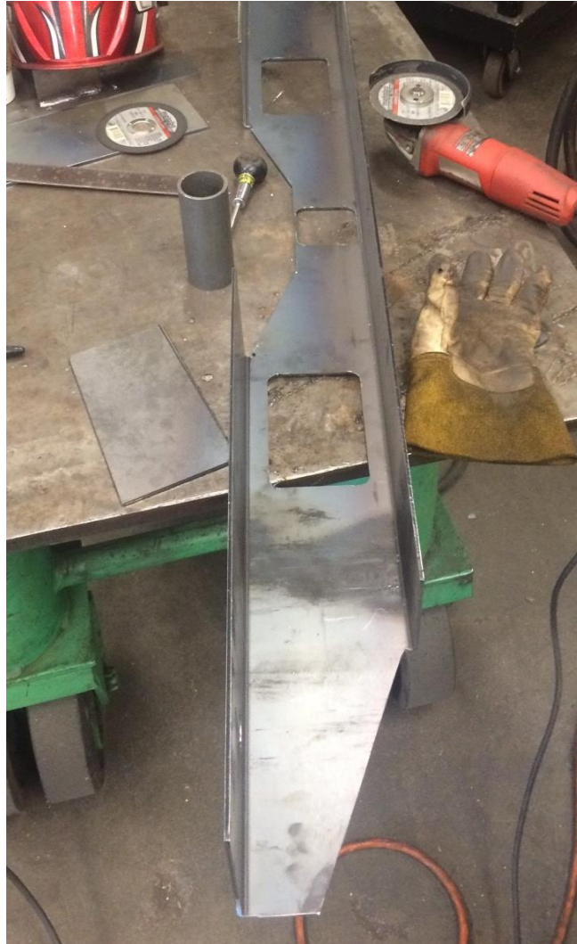
Figure 24. Bent channel of the bumper (back view).
