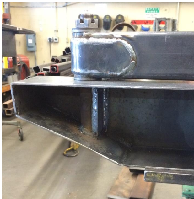
Figure 31. Spindle – hub assembly with spindle welded to bumper and rack installed.
