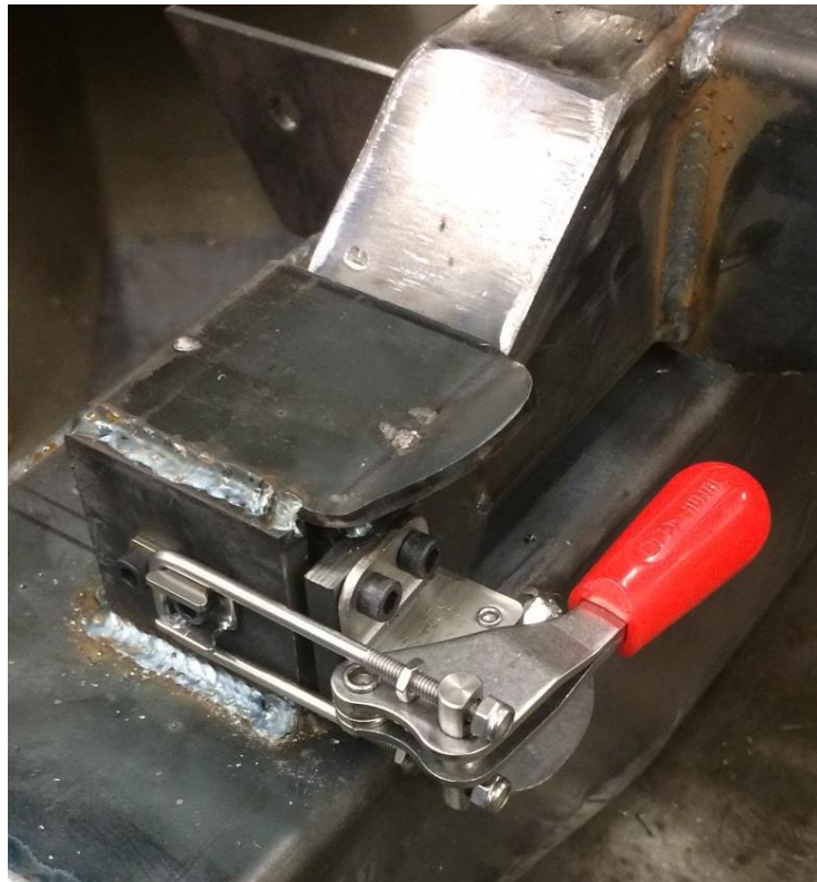
Figure 34. Toggle clamp and latching shelf for the "closed" position.
