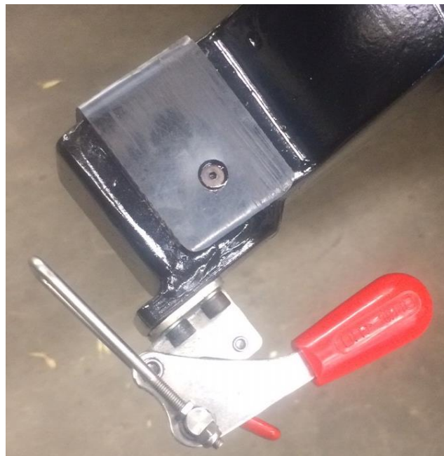
Figure 40. Toggle clamp and Delrin installed.
