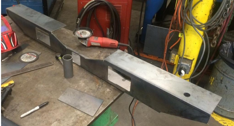
Figure 25. Bent channel of the bumper (top view).
