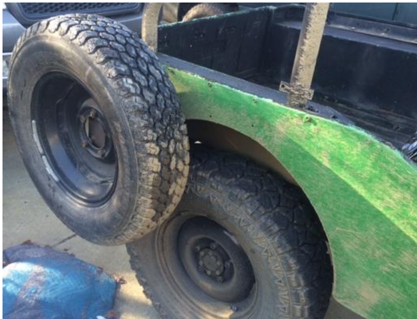
Figure 2. Stock placement of the spare tire on a Willys CJ2A.
