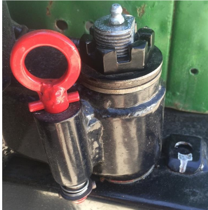
Figure 35. Spring loaded pin and locking ramp for the “open” position.
