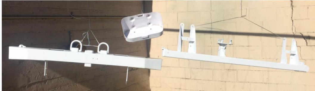
Figure 37. Various parts with a primer coat applied.
