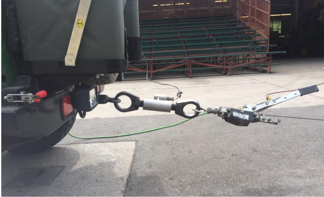
Figure 57. Load cell installed to take force measurements.
