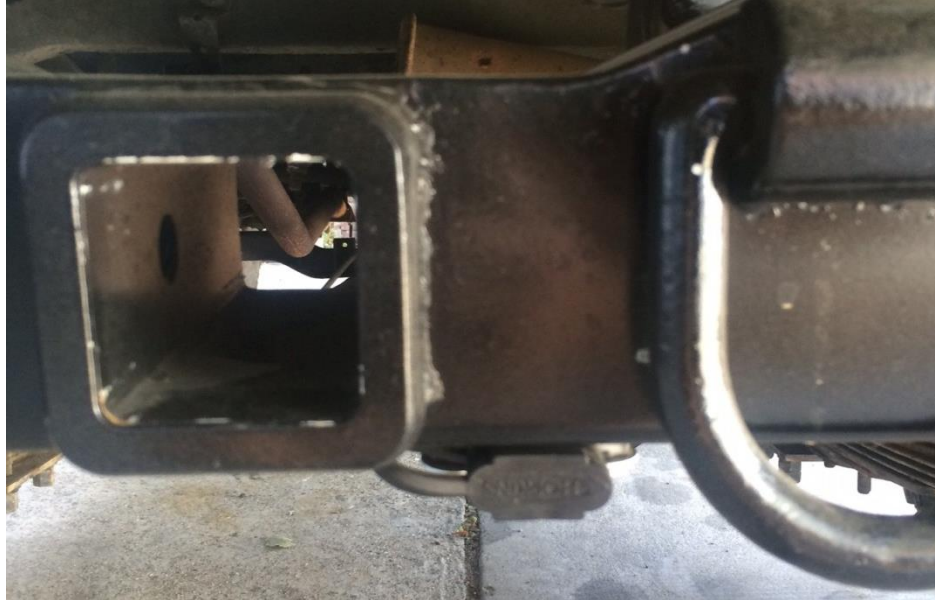
Figure 45. Trailer wiring pigtail installed on bottom side of bumper near receiver tube.
