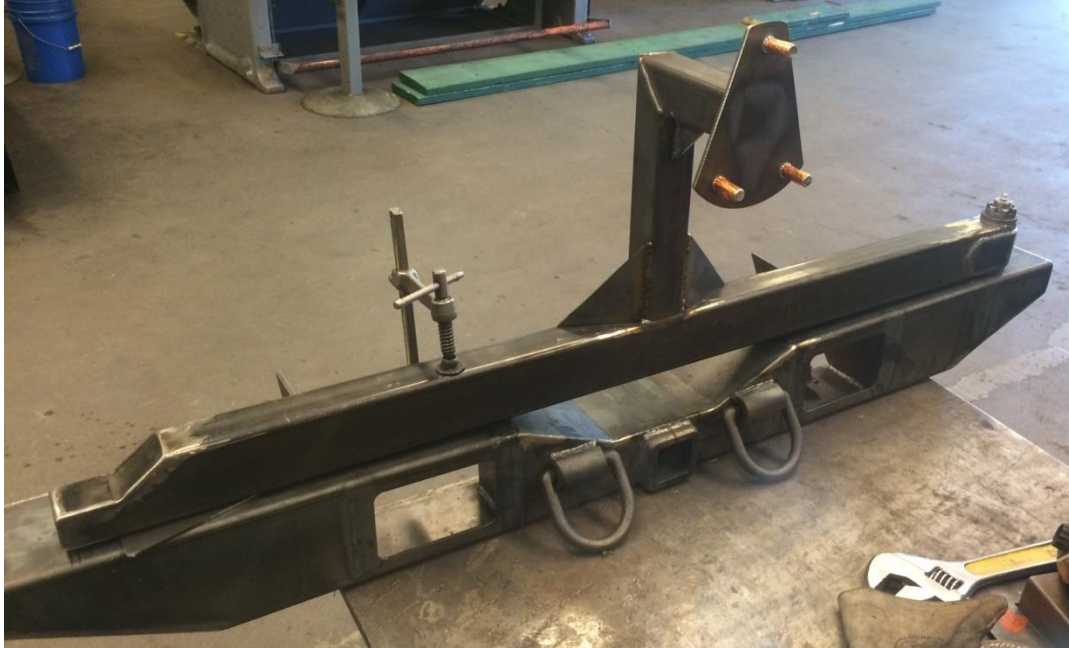
Figure 28. Completed rack placed on top of bumper.
