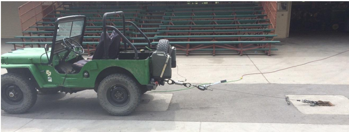
Figure 56. Jeep anchored at back to dead-man via come-along.
