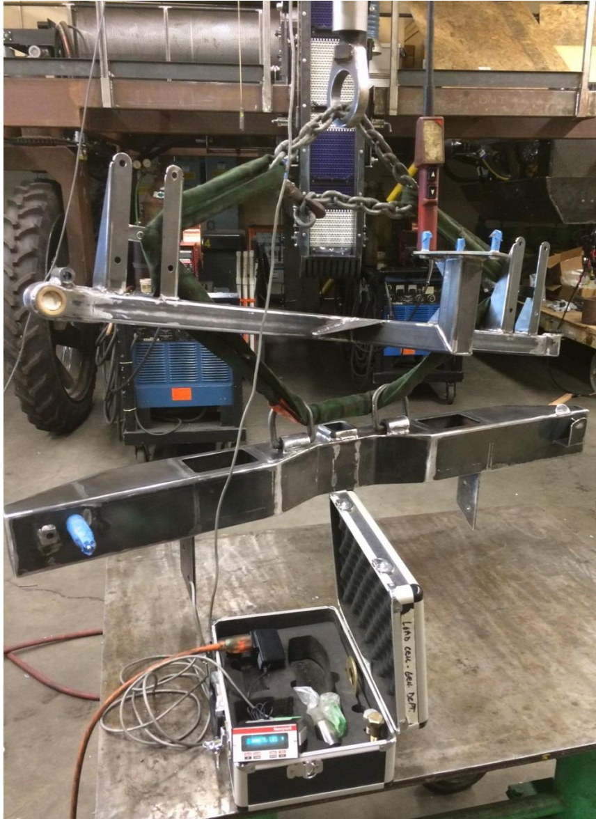
Figure 48. Weighing the new bumper and rack assembly.
