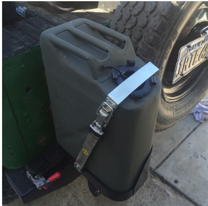
Figure 46. Jerry (fuel) can installed with store-bought tray and strap.
