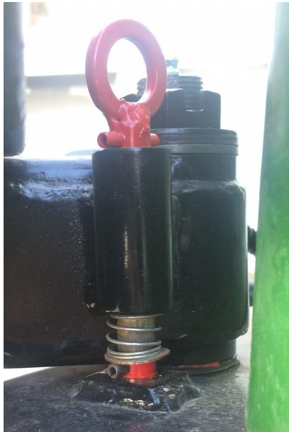
Figure 54. Rack latched in the “opened” position.
