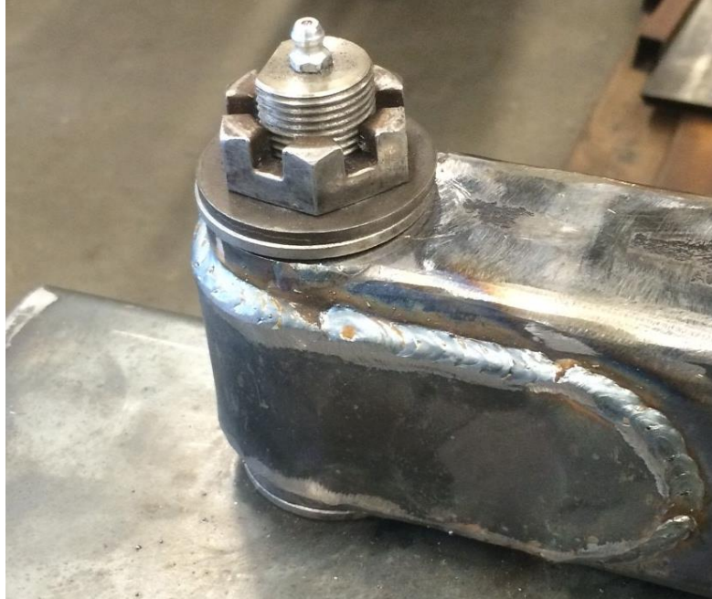
Figure 32. Spindle – Hub assembly with thrust washers, retaining nut and grease zerker visible.
