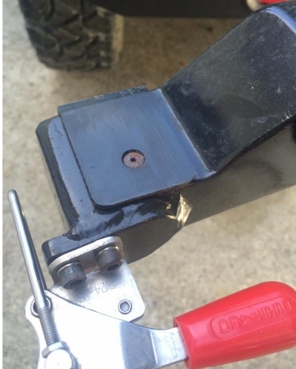
Figure 33. Delrin plastic strip added as a wear surface.
