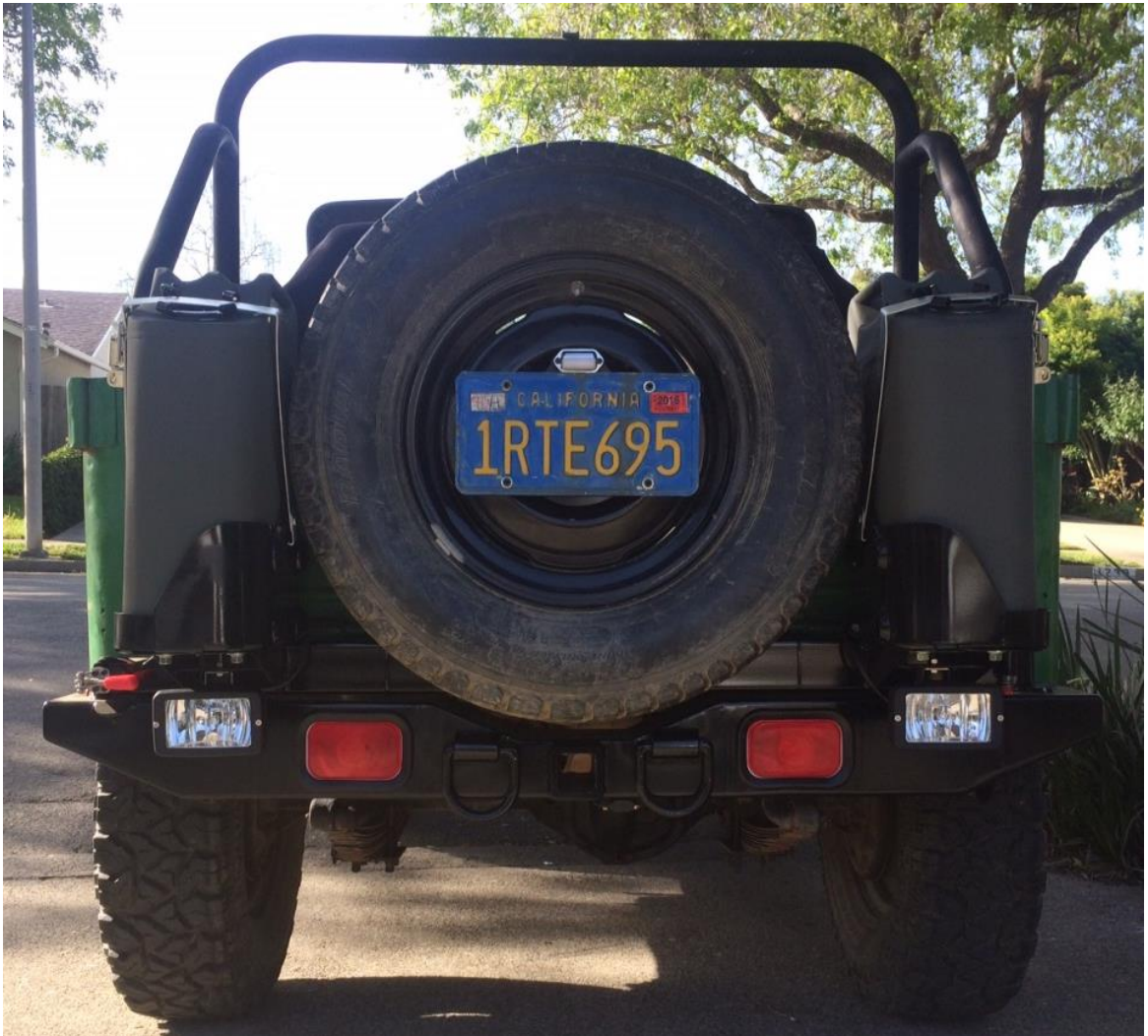
Figure 49. Bumper and rack in “closed” (road transportation) position.
