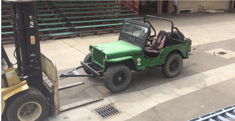
Figure 55. Jeep anchored at front to forklift for applied force test.
