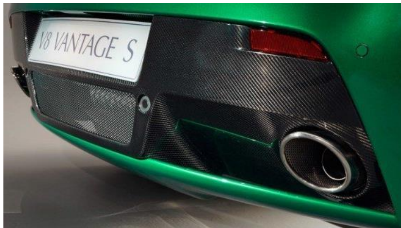
Figure 6. Carbon fiber bumper on a 2011 Austin Martin Vantage S (Top Speed, 2011).
