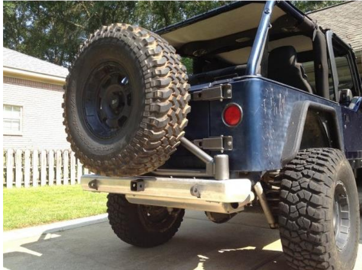
Figure 7. Aluminum bumper with spare tire mount on a jeep (Under Cover Fabworks, 2015).
