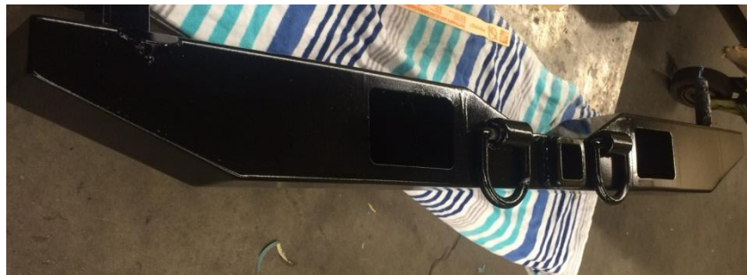
Figure 38. Bumper with its final coat of black paint dry.
