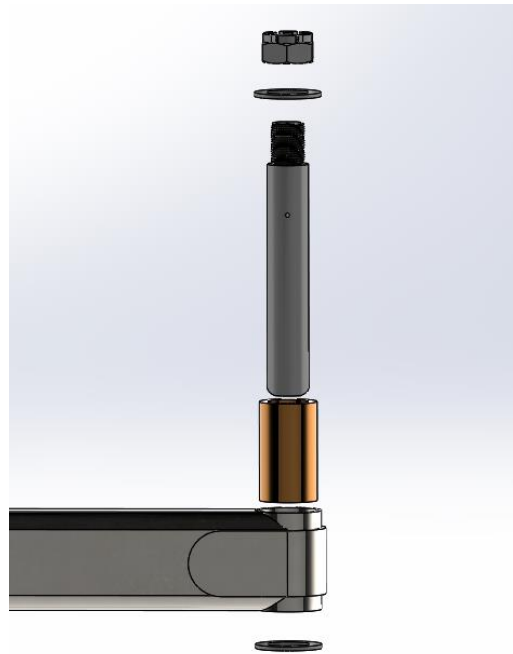
Figure 19. Exploded view of the spindle-hub assembly.
