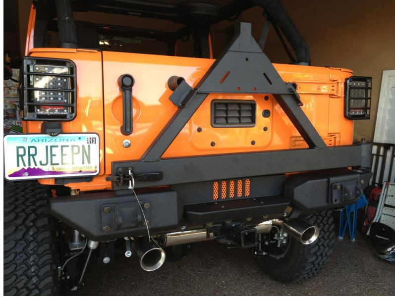
Figure 8. A steel bumper with spare tire mount installed on a modern jeep (Rugged Ridge, 2015).
