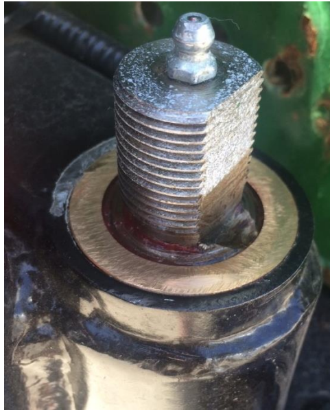
Figure 30. Spindle – Hub assembly with bushing installed.
