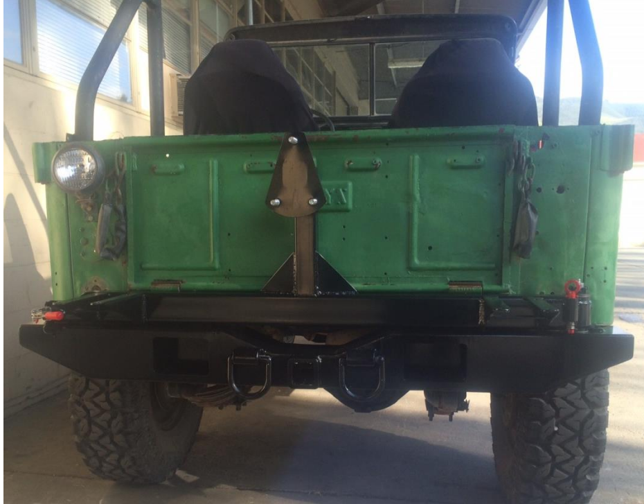
Figure 41. Bumper and Rack assembly installed.
