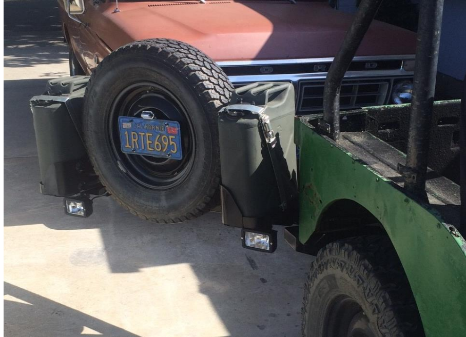
Figure 53. Rack in “open” (tailgate access) position.
