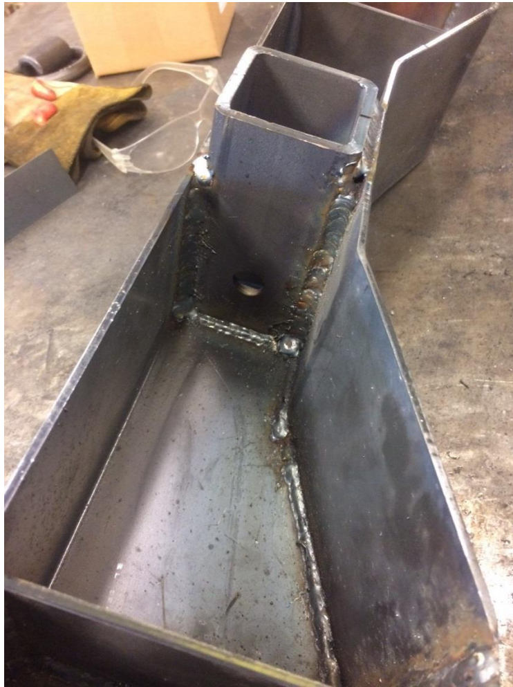
Figure 27. Receiver tube welded into bumper channel.
