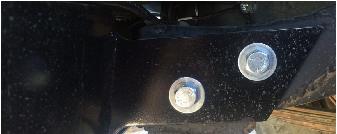
Figure 42. Bumper mounting plate bolted to frame.
