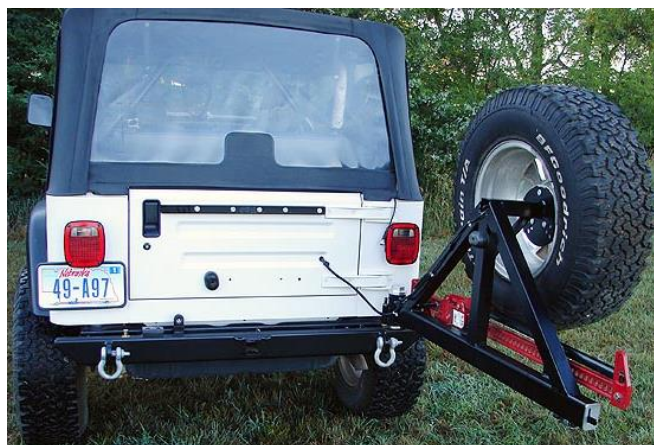
Figure 4. An aftermarket bumper and spare tire rack currently produced by 4x4 Group Buy (2016).
