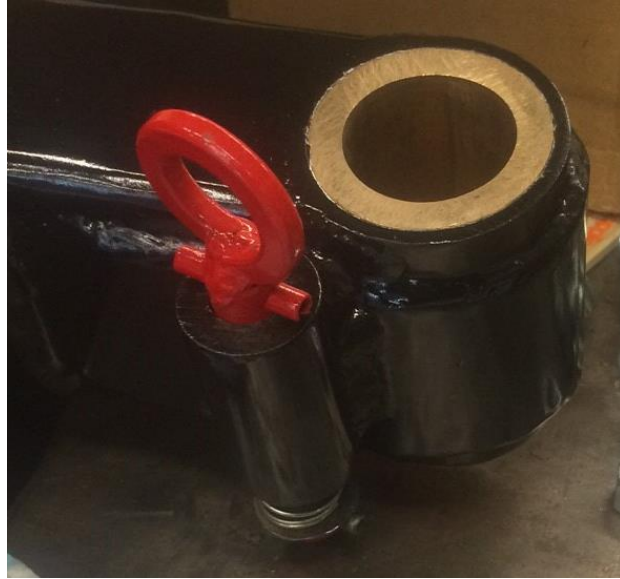
Figure 39. "Open" position latch installed.
