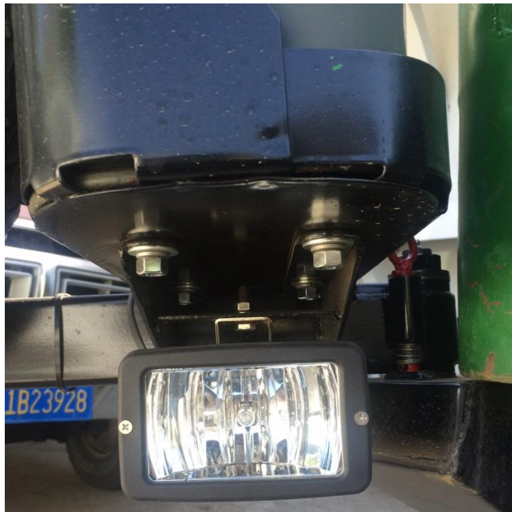
Figure 44. Flood light installed on rack below Jerry (fuel) can.
