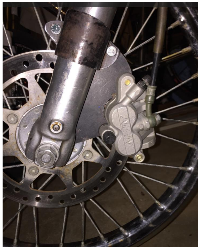
Figure 20: Caliper and Mount Installed On 1973 Yamaha CT3
