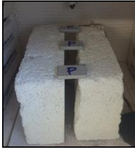
Figure 11. Furnace set-up for the Production heat treatment. The samples were placed at a minimum of one inch apart per AMS 2770 and raised to the center of the furnace using refractory bricks.
