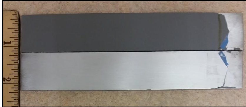
Figure 4: Non-etched 7075 coupons after wedge testing show that epoxy only remains adhered to one face instead of being split between both faces.
