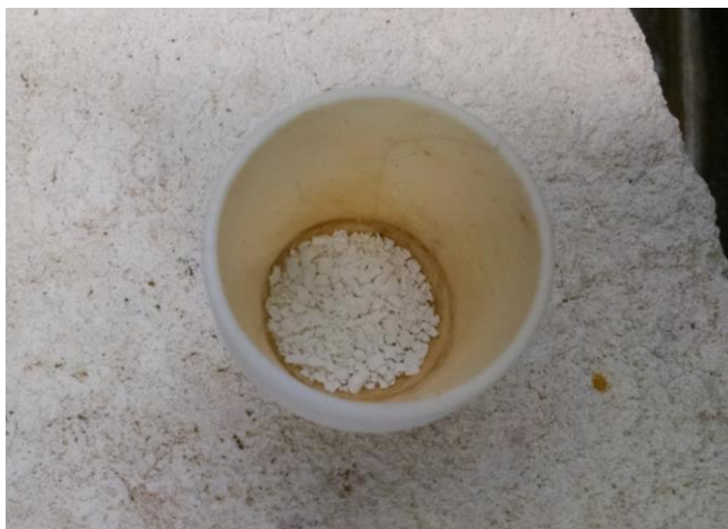
Figure 5. The MgO clumps together in flakes. Agitation of the flakes breaks them up into a fine powder.
