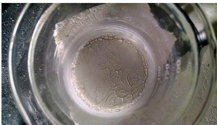
Figure 4. Dry magnesium hydroxide on the bottom of the beaker after oven drying.
