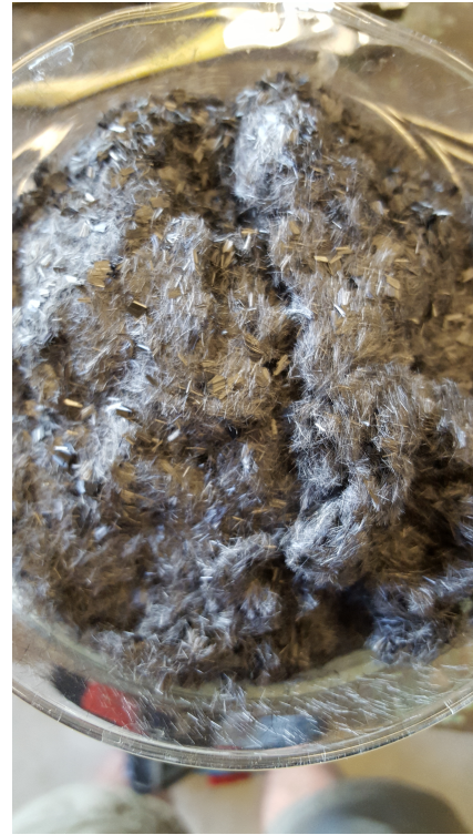
Figure 5 – Carbon fibers that are nearly dried with a few bundles remaining.
