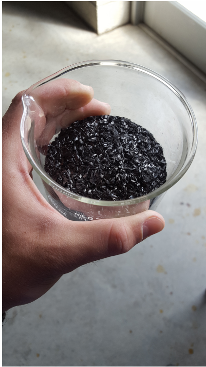
Figure 4 – Carbon fibers as received in fascicular bundles prior to drying.
