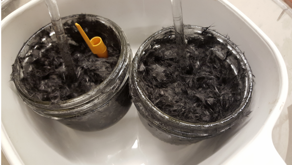
Figure 6 – Prepared samples of carbon fibers in silicone oil.
