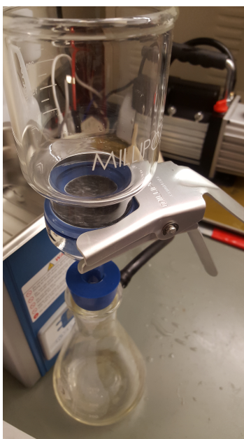
Figure 8 – Vacuum filtration process with ultrasonication bath in background on the left.
