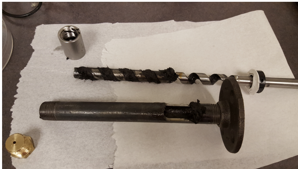
Figure 7 – Screw and chamber of the Filastruder with carbon fiber and oil during preliminary tests.
