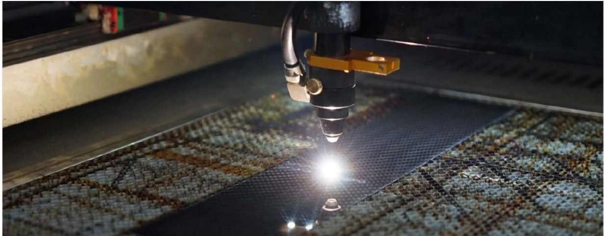
Figure 4 - Image of the CO 2 laser ablation process Common Fibers uses to manufacture their composite hinge technology.
