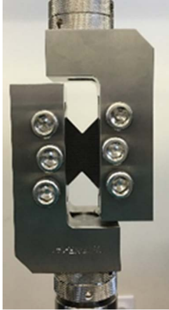
Figure 10 - Image of the ASTM D7078 fixture with specimen loaded ready to be tested.
