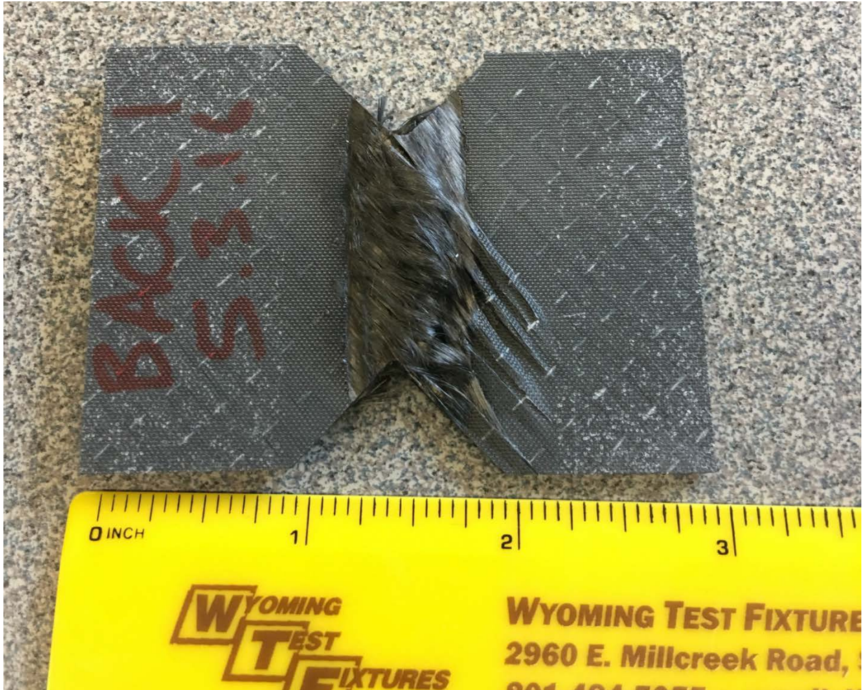
Figure 21 - Image of a [+45/-45/0]_s hinged laminate post V-Notch shear testing. The image displays the failure mode of splintering delamination along the hinge-composite interface.
