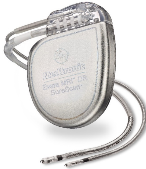
Figure 2: Example of a common ICD. Can and electrodes are shown
