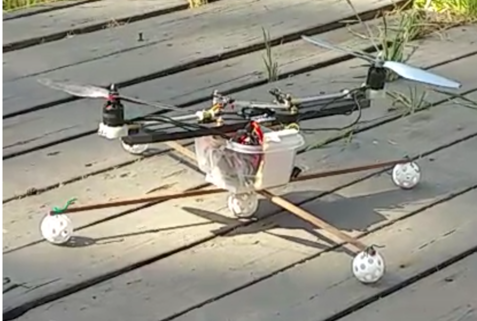
Figure 3: Completed Tilt Rotor Drone with Landing Pad
