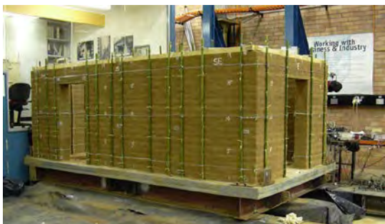
Figure 9: Bamboo reinforcement full scale testing
