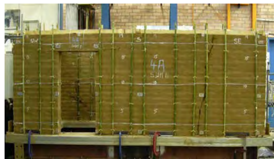
Figure 10: Bamboo reinforcement full scale testing - Elevation
