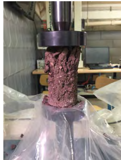
Figure 18: Results of testing cylinders
