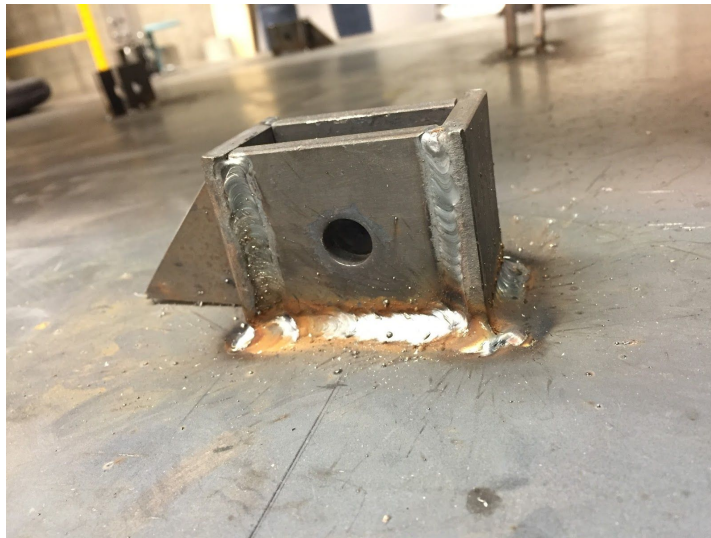
Figure 1: Completed interior clevis welded to the baseplate.
