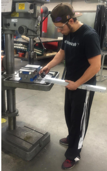
Figure 6: Having to remove plug to drill holes
