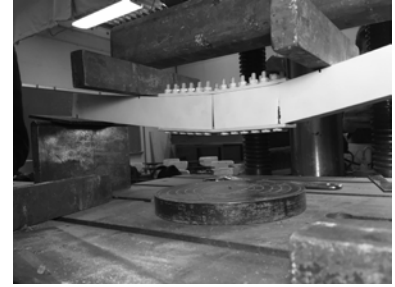
Figure 4: Moment Connection Test
