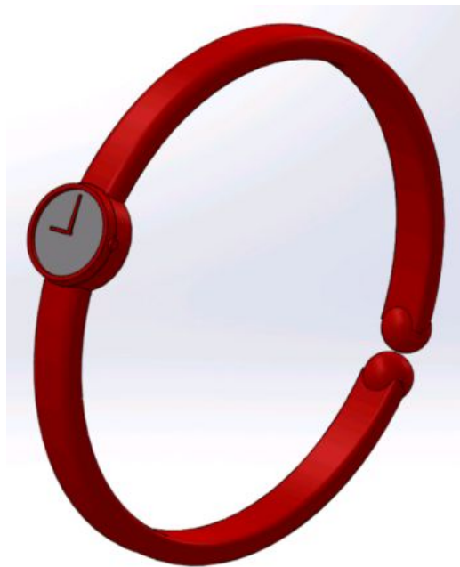
Oluso CAD design with discrete panic button
