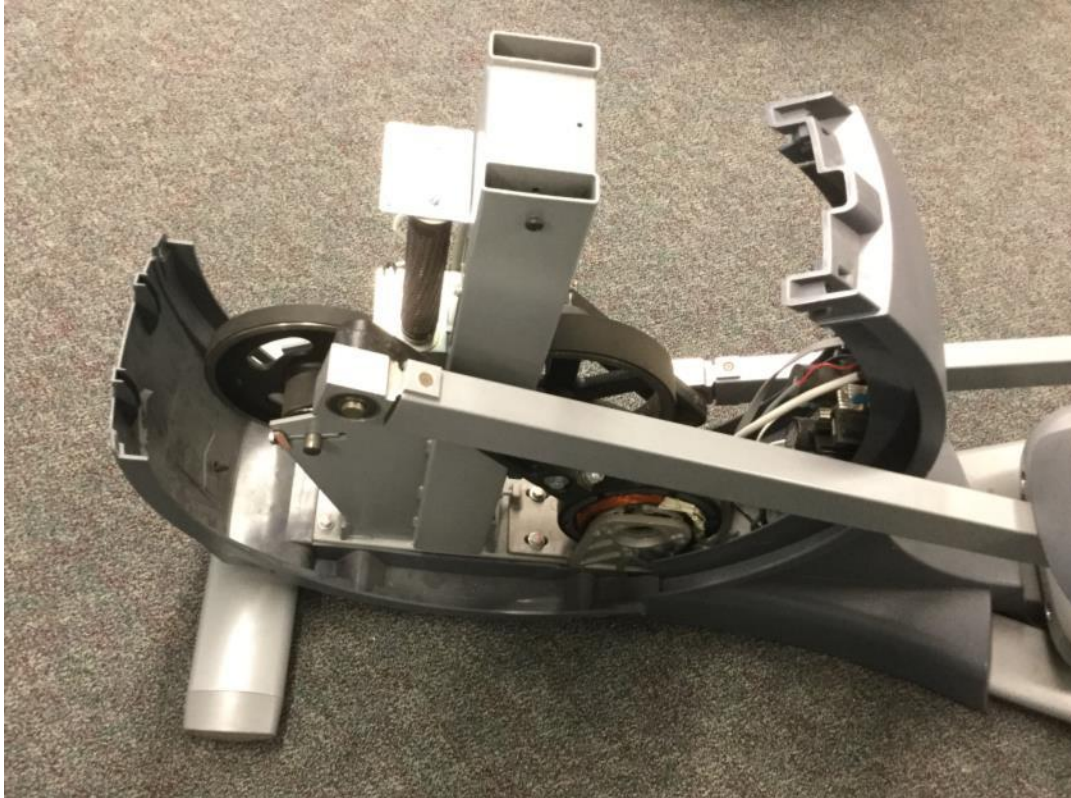
Figure B-3: Rear elliptical housing top panel removed
