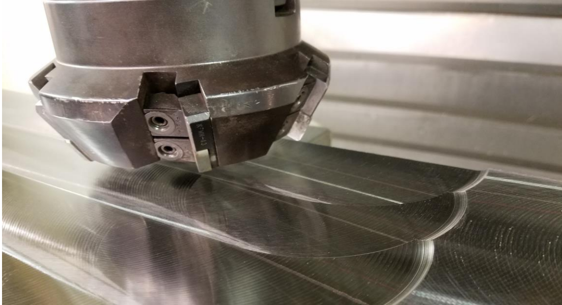
Figure 23. Tapered face mill used to face bolster plate.
