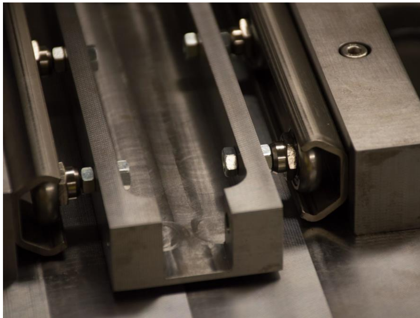
Figure 29. Nuts protruding into slot of pulley v-block.
