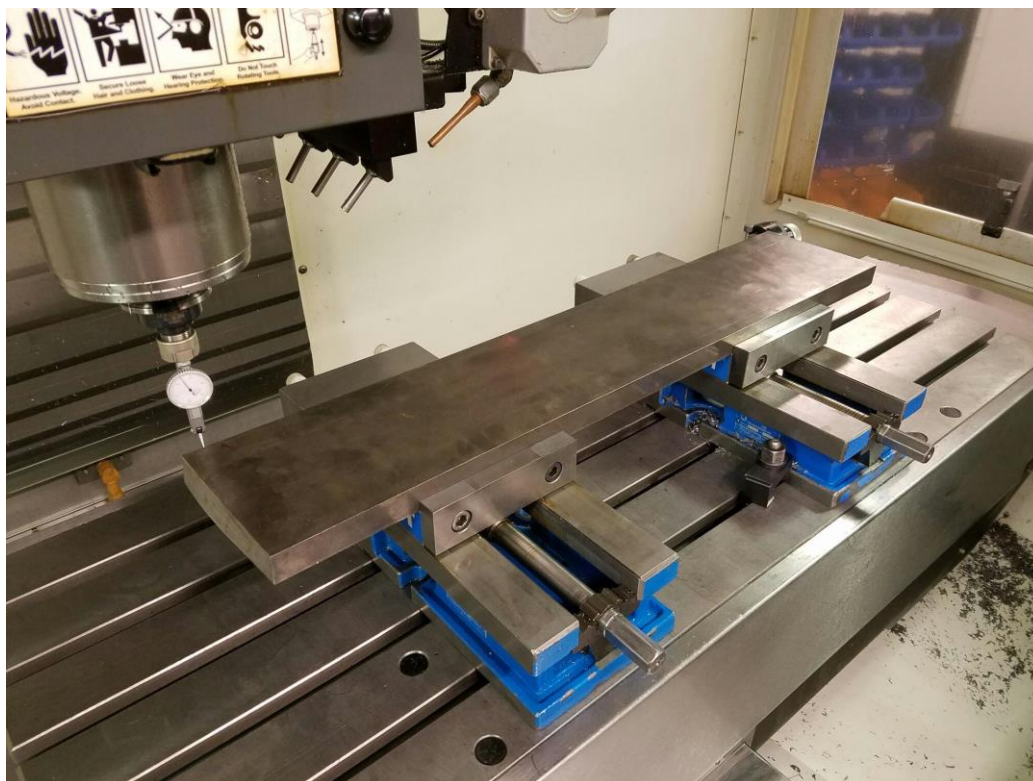
Figure 22. Bolster plate milling setup.
