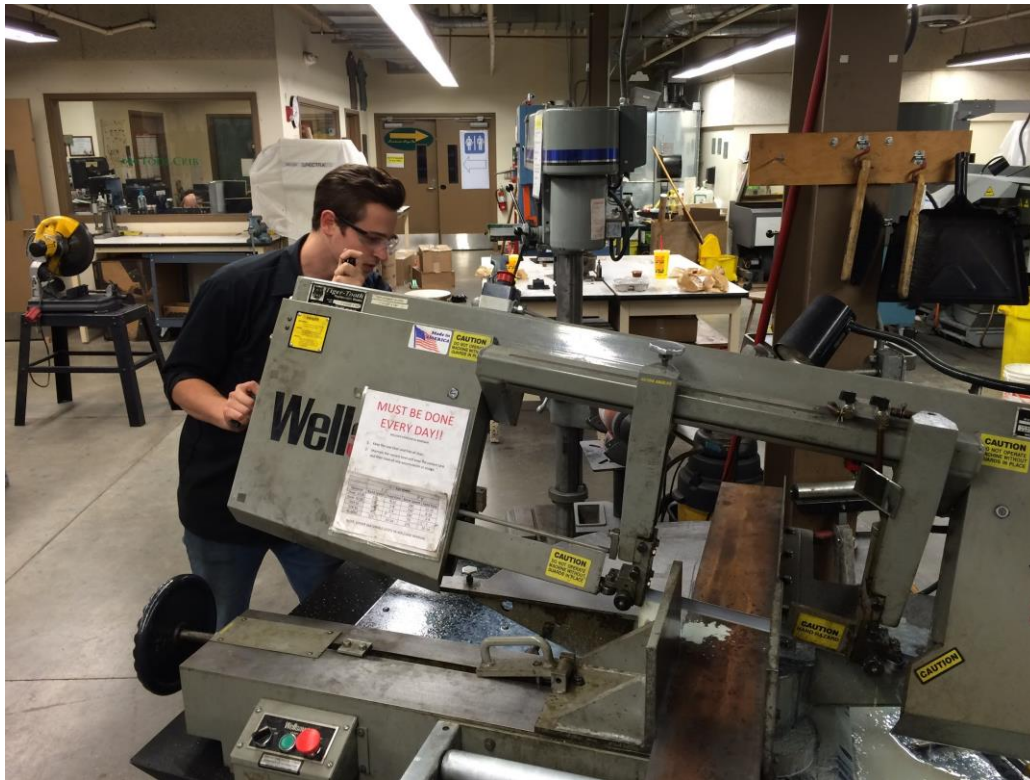
Figure 21. Cutting steel extrusion to length.
