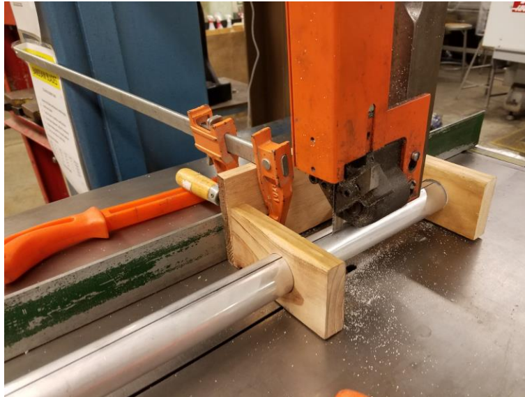
Figure 27. Aluminum tubing being cut on the vertical band saw with a custom wood fixture used to maintain proper orientation.
