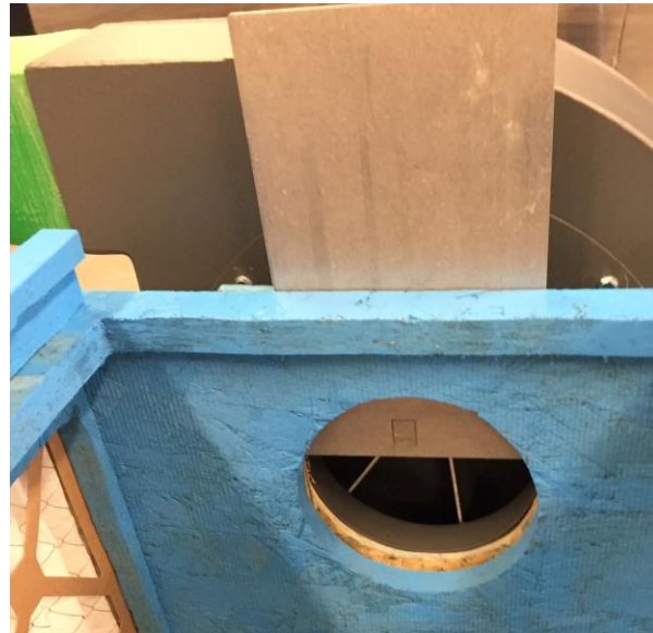
Figure 18. The gate valve restricts airflow into the blower, shown half-open.
