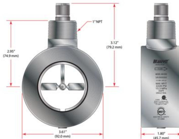
Figure 16. Dimensioning of Gas Quiksert B142-20M
