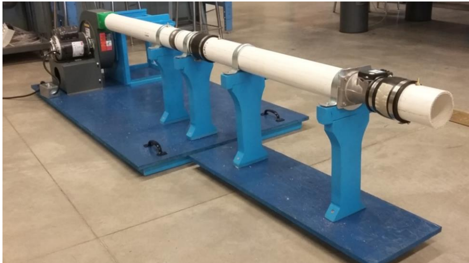
Figure 23. Test rig set up with MAF section attached.
