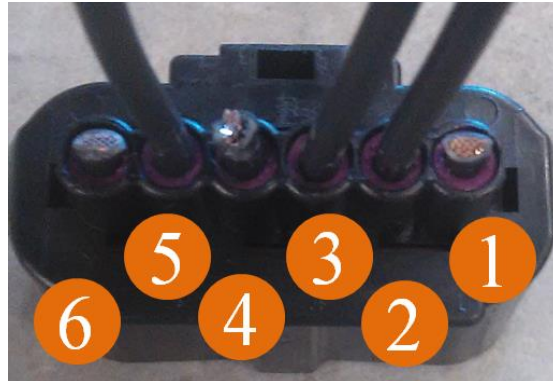
Figure 20. MAF Sensor Circuit Description.
