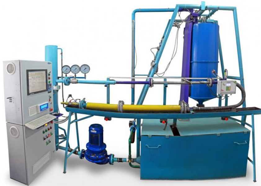
Figure 2. Example Setup for a Prover type calibration. (Courtesy of EnergoFlow)
