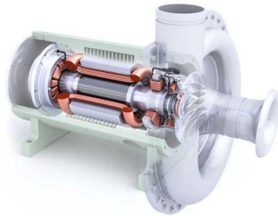
Figure 1.1. (a) Industrial full-size radial magnetic bearing. (b) SKF AMB assembly in an industrial water pump.
