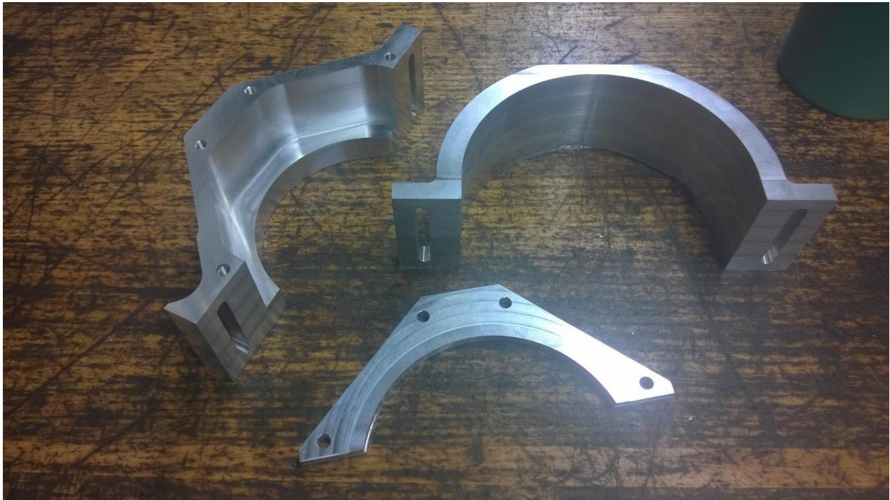
Figure 12.2. CNC milled, aluminum, stator case components.
