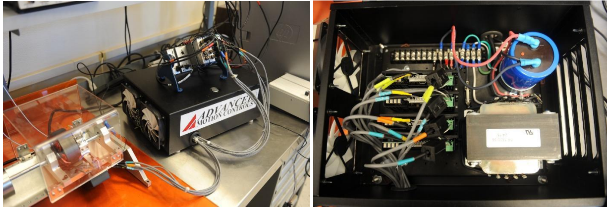
Figure 12.7. Left: Electronic enclosure with wire connections to the AMB and NI FPGA Controller. Right: Inside of electronic enclosure with the four servo drives mounted to the power supply.
