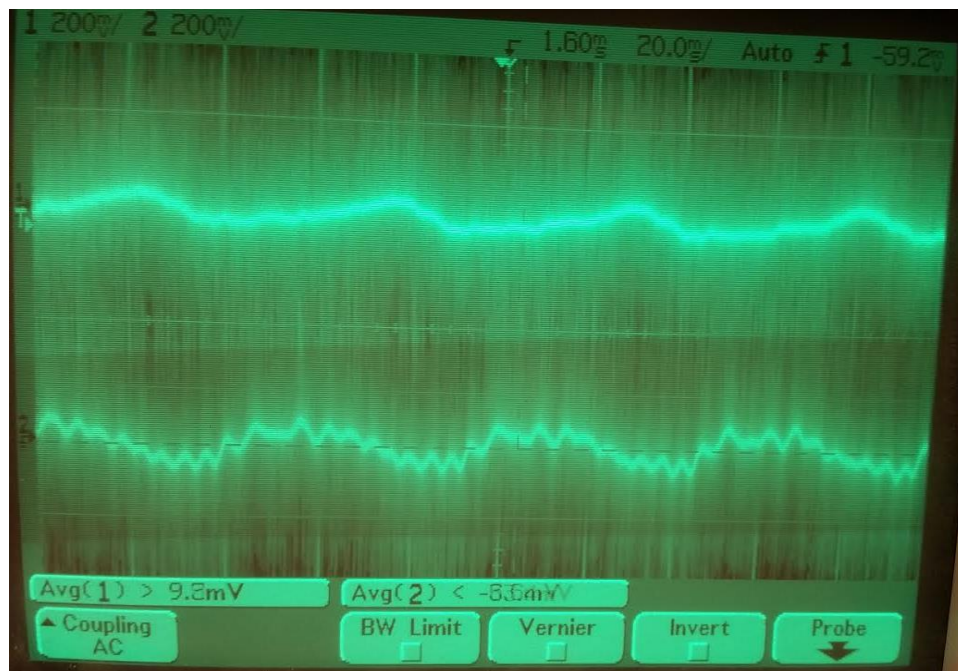
Figure 16.2. Position probe outputs at 1,000 RPM with AMB applying active feedback.
