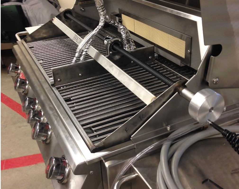
Figure 7: Completed testing apparatus with insulated wires in the provided natural gas grill.
