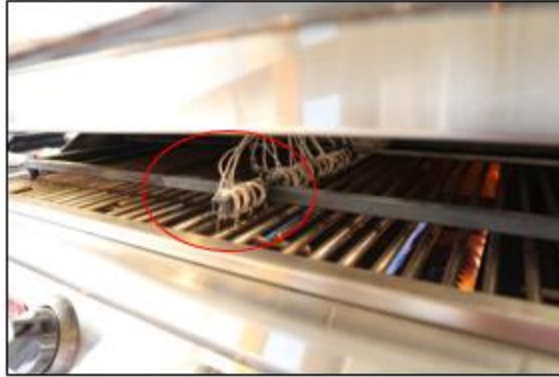
Figure 2: Team License to Grill's testing apparatus Highlighting the method of attaching thermocouples.
