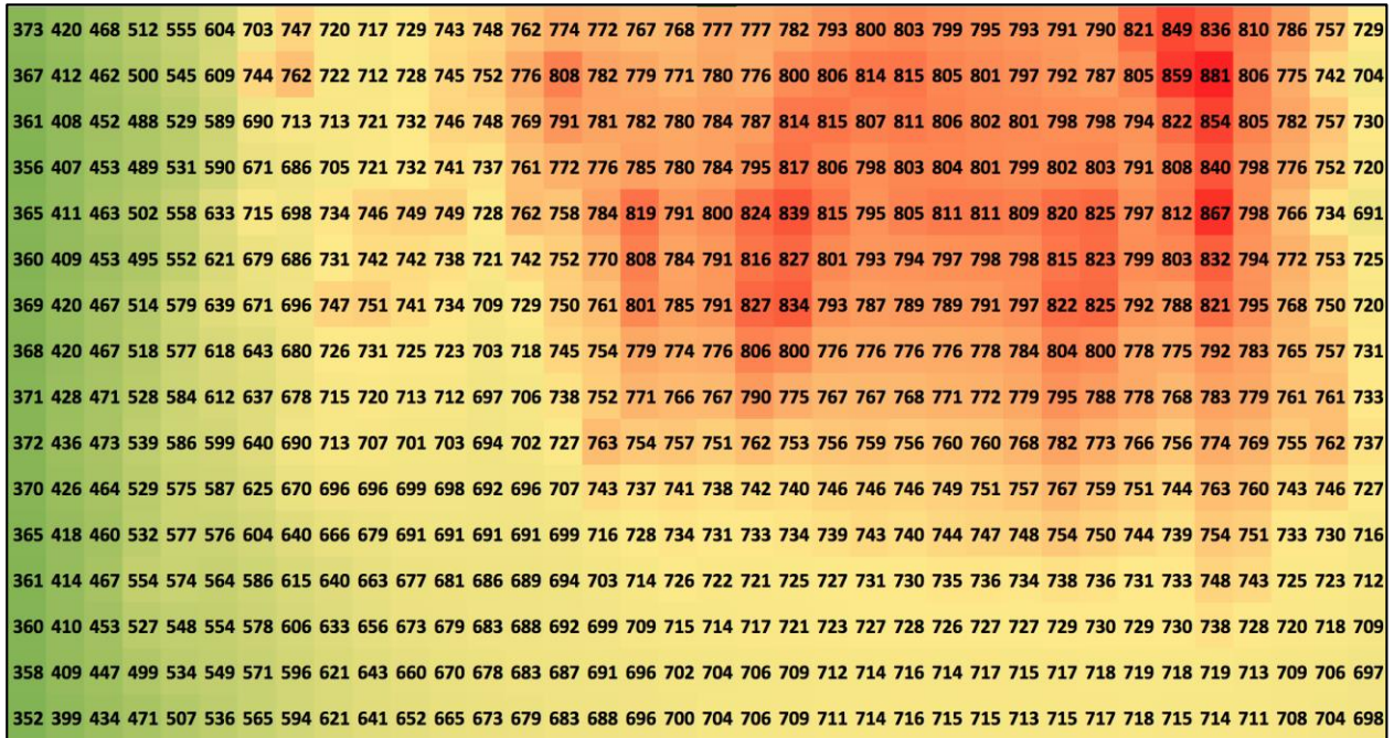
Figure 10: Grid of average temperatures with color mapping for visual representation of Test Run-1.
