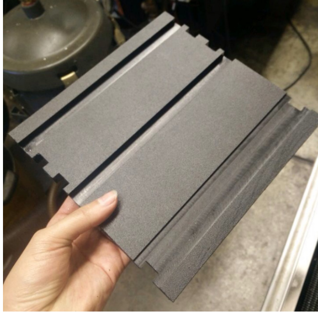
Figure 15. Base plate with machined grooves and dovetail joints.
