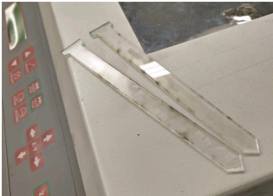
Figure 20. Positioning tools after machining. The black spots are areas that the laser burned. They do not affect the operation of the positioning tools and actually provide a better visual guide to line up the flipper.
