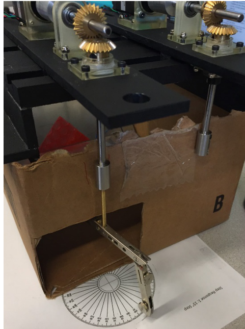
Figure 25. Dry step and frequency response test using angle indicator and printed protractors
