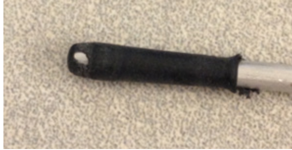
Figure 11. Plasti-dip damage after repeated installation
