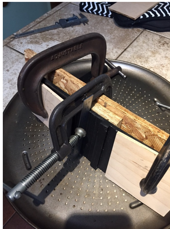
Figure 24. Attempting to unwarpage the planks by clamping them down and putting them in the oven.
