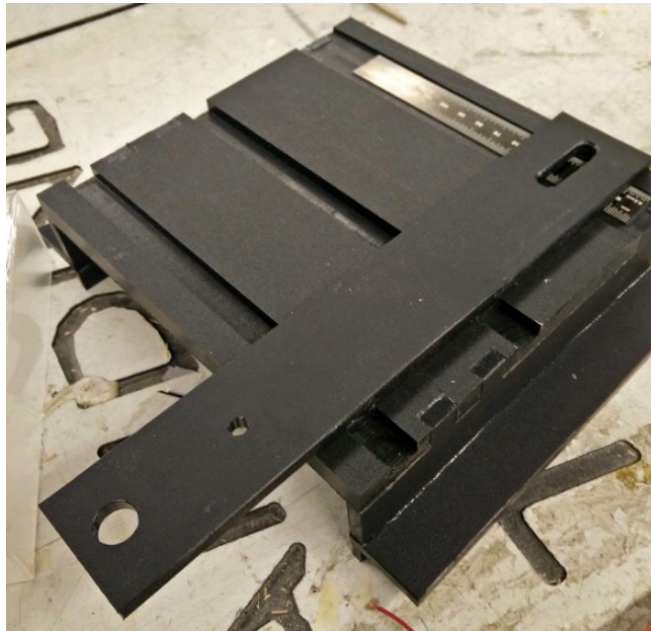
Figure 16. Fully-assembled base plate with supports after being epoxied. The ruler had not yet been epoxied onto the rig. The motor planks have holes drilled for the vertical shaft and positioning tool.
