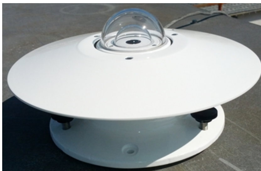
Figure 15. Eppley Pyranometer used for measuring solar intensity
