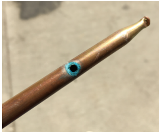
Figure 10. Close up of the hole used to drain, flush, and refill the heat pipe
