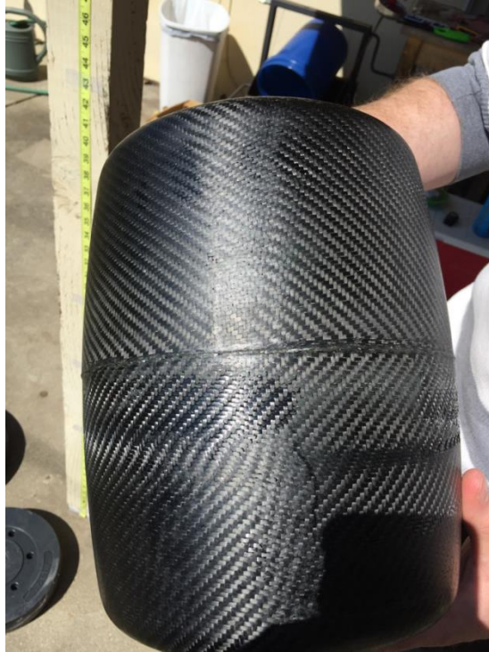
Figure 51: Close-up side view of canister #3 post impact
