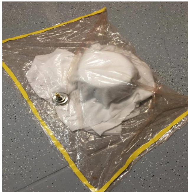
Figure 19: Debulking the mold
