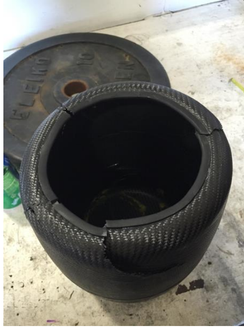
Figure 40: Canister #1 additional top view post-impact
