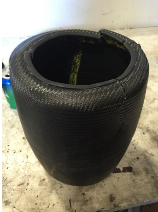
Figure 38: Canister #1 top view post-impact
