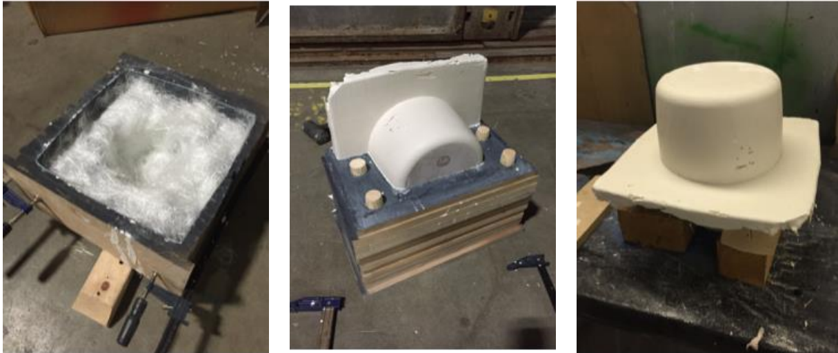
Figure 16: Strands of fiberglass placed into the mold cavity (left), the post cured mold with one half of the MDF mold removed (middle) and the resulting plaster mold (right).
