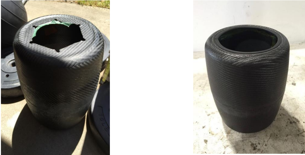
Figure 33: Excess carbon at the inner lip of the canister (left) was trimmed to the proper diameter shown (right).
