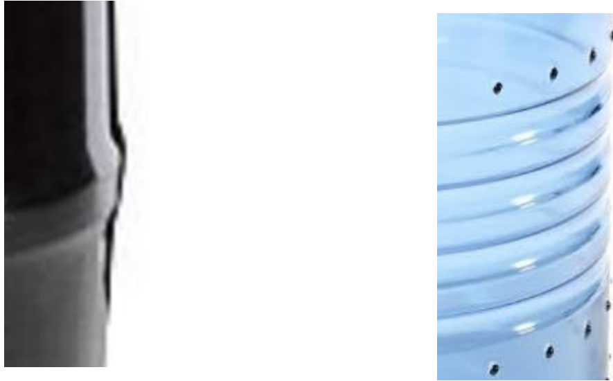
Figure 58: The Garcia (left) and Bear Vault (right) both exhibit geometric features which make the middle hoop section the stiffest section of the canister. By applying more ABS plastic on the Garcia the bending stiffness is greater. The BV has a ridge feature at the center increasing the moment of inertia of the cross section in the hoop direction.
