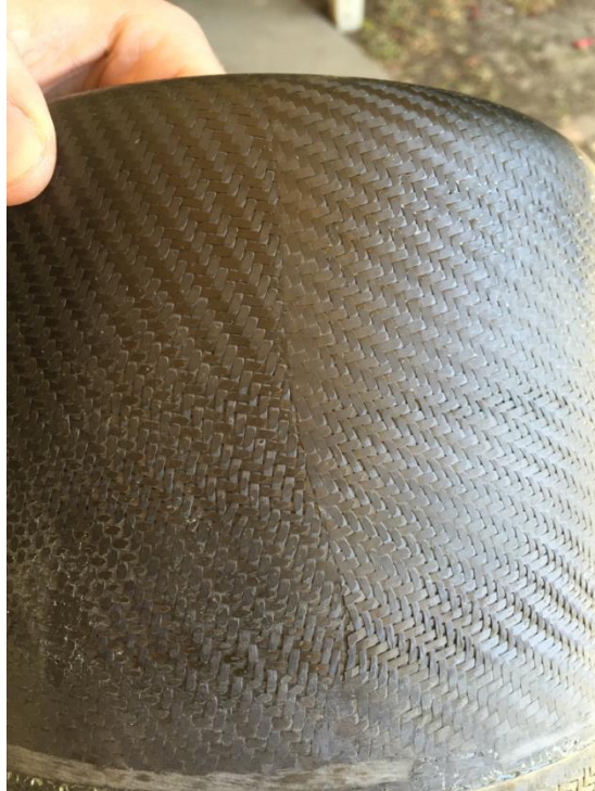
Figure 46: Close-up view of crack on canister #2
