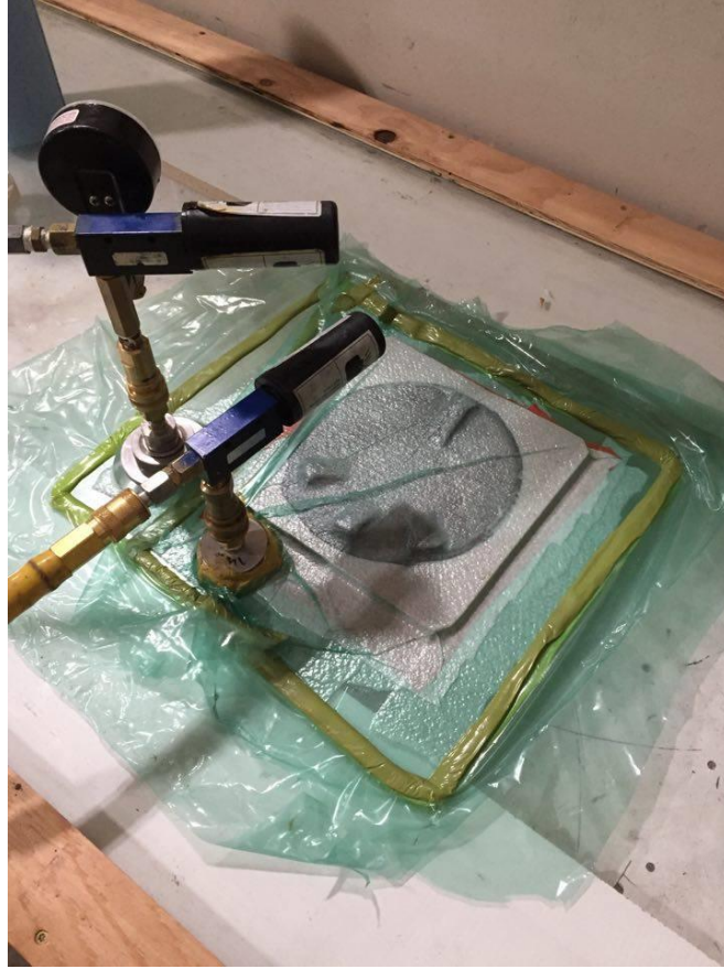
Figure 31: Vacuum bagging process to cure wet layup of carbon fiber lids.
