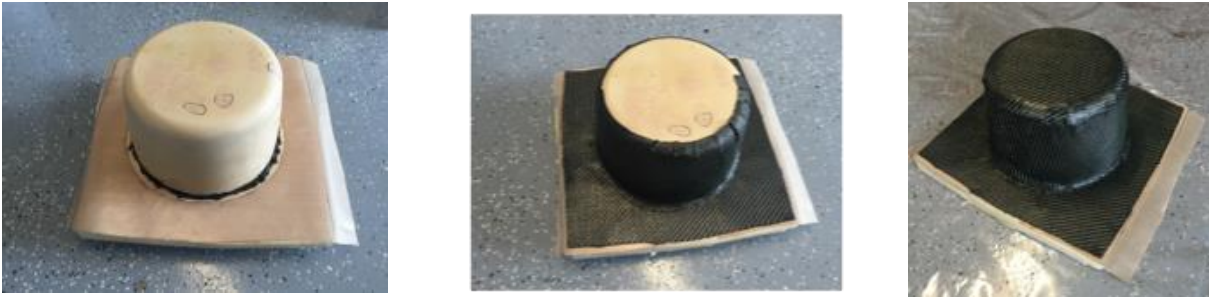
Figure 18: Application of prepreg to the plaster mold. Stencils were applied in the order shown, from left to right.
