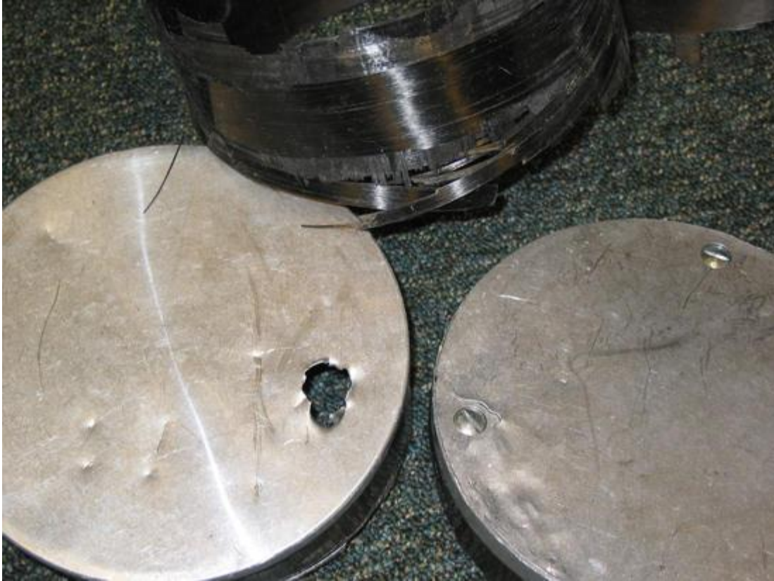
Figure 60: Bearikade which broke from an encounter with a brown bear.
