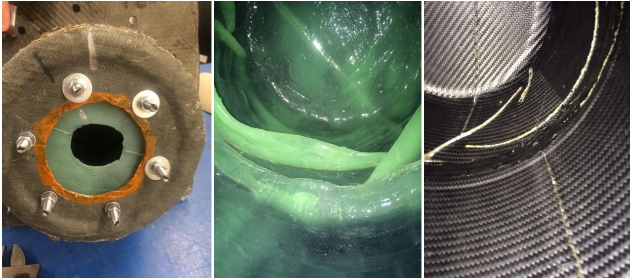
Figure 28: Top portion of the mold post cure with the aluminum plate removed (left). The bag exhibited wrinkling in certain portions of the canister (middle). This lead to wrinkled carbon on the interior of the canister (right).
