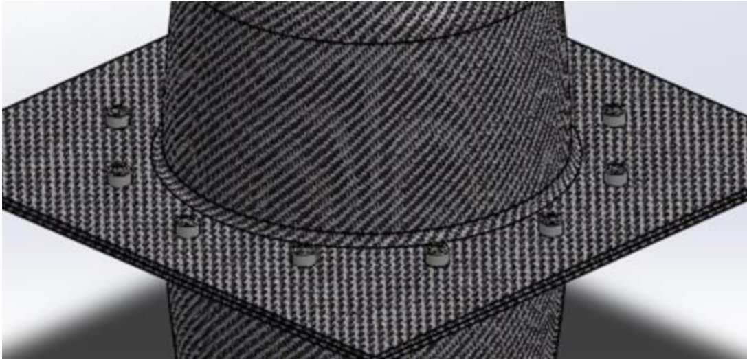
Figure 12: Middle-section of carbon mold with circular bolt pattern.
