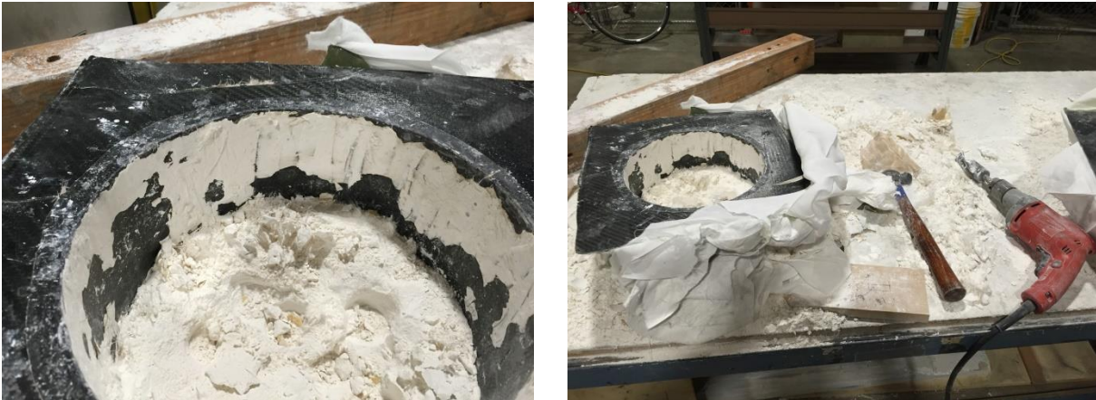
Figure 21: Removal of the plaster from the carbon molds post cure with destructive practices.
