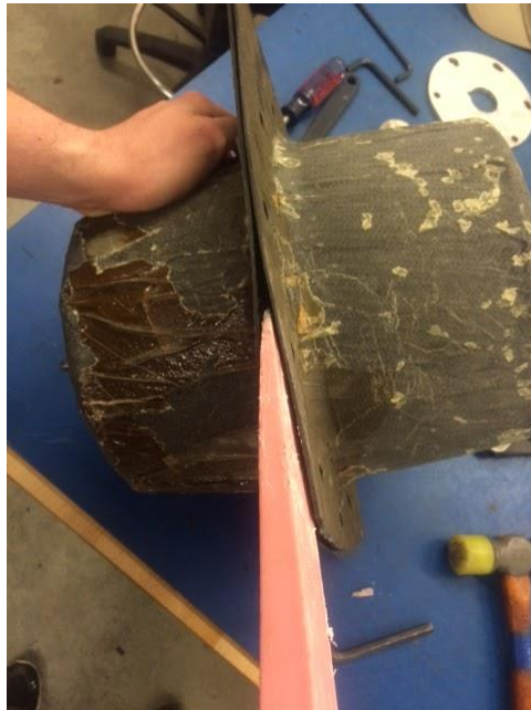
Figure 29: Wedge inserted between flanges to remove one half of the mold from the bear canister.
