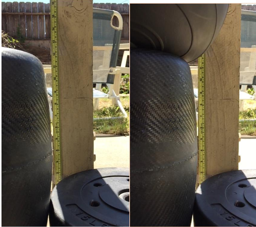
Figure 41: Top before and after deflections for canister #2
