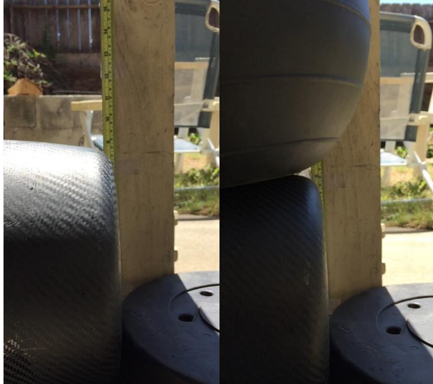
Figure 42: Side before and after deflections for canister #2
