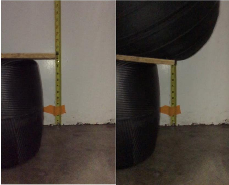
Figure 36: Top before (left) and after (right) deflections for canister #1
