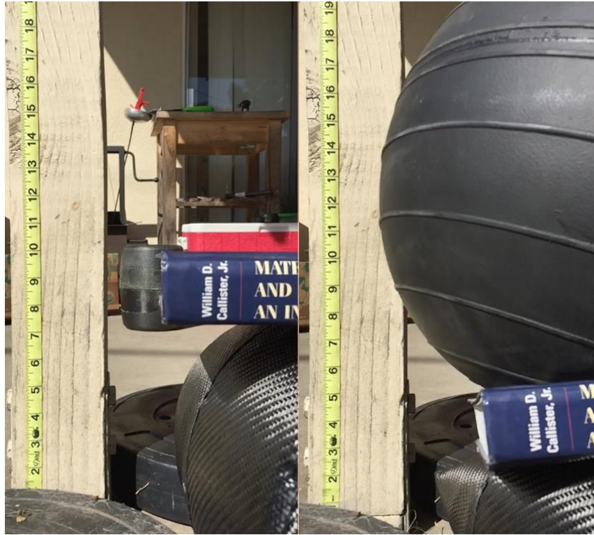
Figure 54: Side before and after deflections of canister #4
