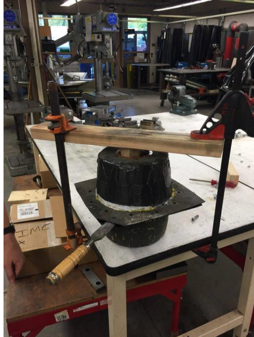
Figure 30: Jig used to remove the top half of the mold from the canister.
