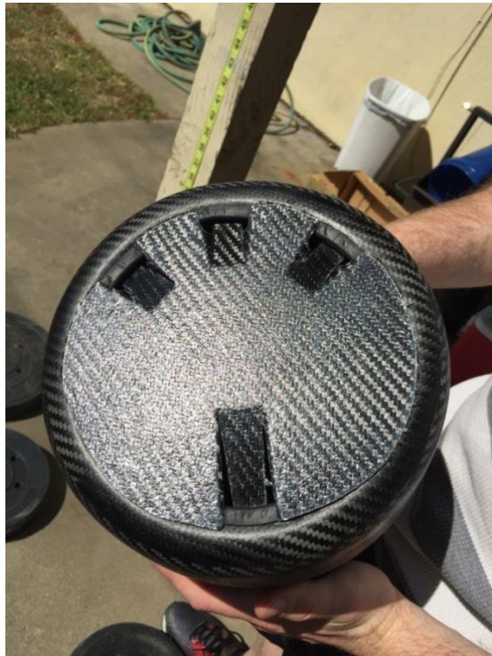
Figure 52: Close-up top view of canister #3 post impact
