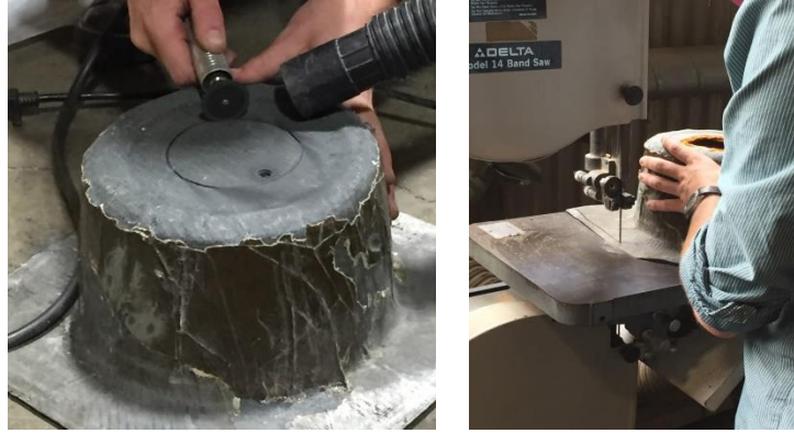
Figure 24: The access hole for the vacuum connector was cut into the top of the mold using a handheld router with a cutting wheel (left). The flange contained sharp edges, which were trimmed for safe handling (right).
