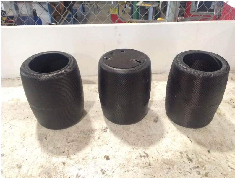
Figure 34: Three of the four manufactured canisters. On the left: the first, middle: third, right: fourth. Using varying layups and lamination techniques, the cans had differing lamination qualities. Only the First
