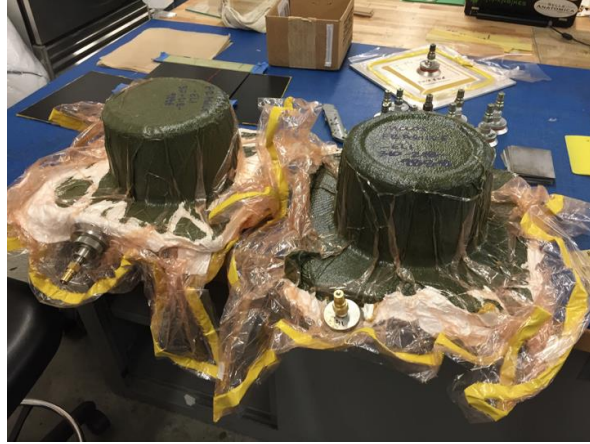
Figure 20: Carbon molds after cure cycle in autoclave.
