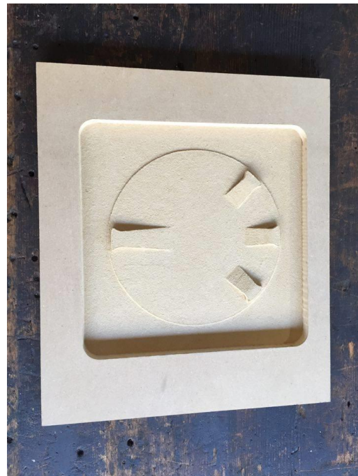
Figure 32: MDF mold for creating lids with integrated tabs.
