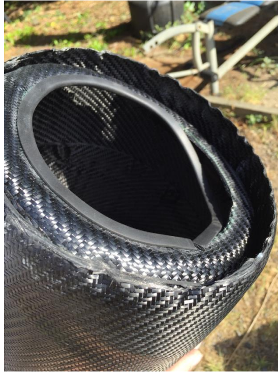
Figure 57: Top-side view of canister #4 post impact
