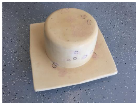
Figure 17: Plaster mold with depressions filled and imperfections sanded to a wet finish.
