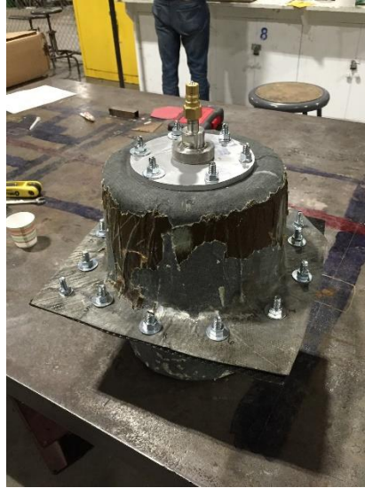
Figure 26: Assembled bear canister mold with all accessory components installed.
