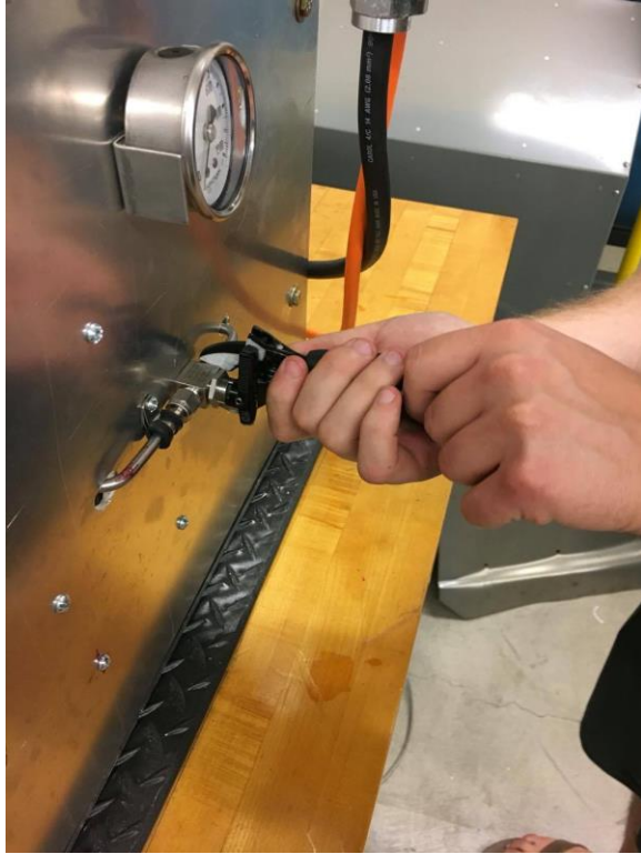
FIGURE 28. INSTALLING AND TIGHTENING A SWAGELOK FITTING
