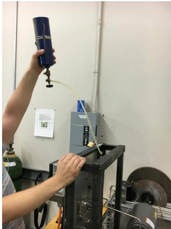
FIGURE 30. USING THE VESSEL TO CHARGE THE SYSTEM
