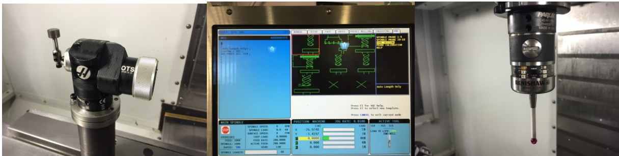
Figure 24 (L to R): Renishaw OTS, Tool Offset Screen, Renishaw OMP40-2
