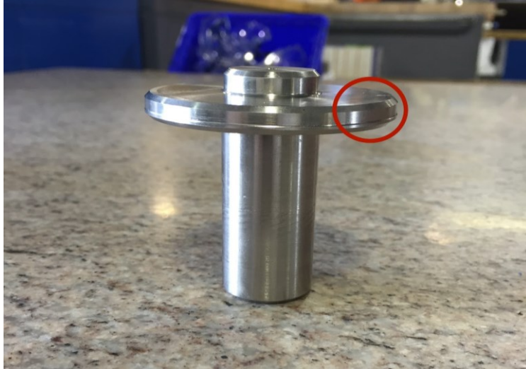
Figure 28. Mill Fixture Defect
