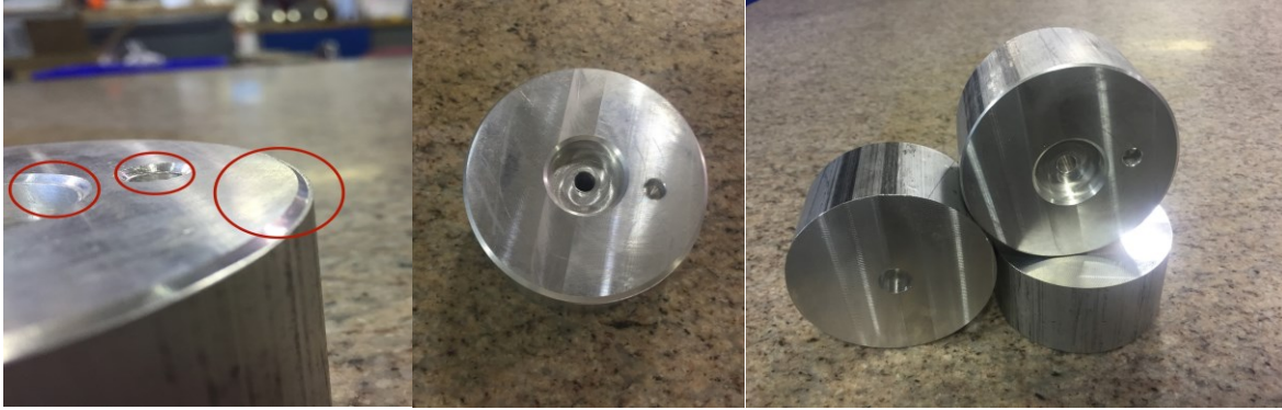
Figure 30: Chamfer Defect vs. Final Mill Blank
