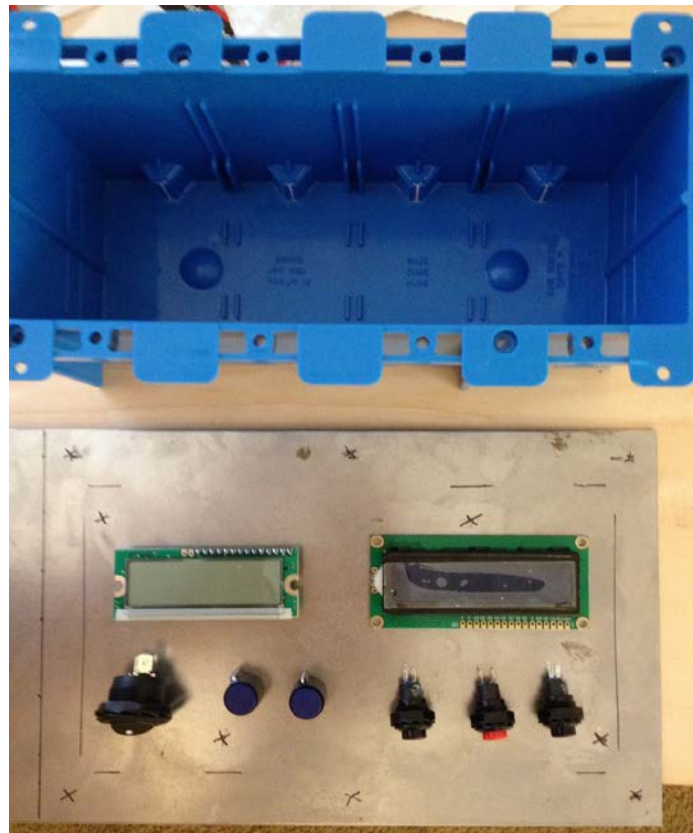
Figure 4.17: Materials for Control Circuitry Housing
