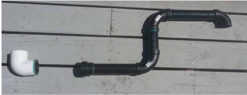
Figure 4.2: AC Pump Plumbing (Preliminary Model)
