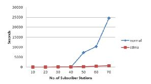
Fig. 4. Total end-to-end delay for Comparison 1
