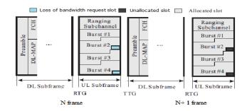
Fig. 1. "Loss of bandwidth request" incident
