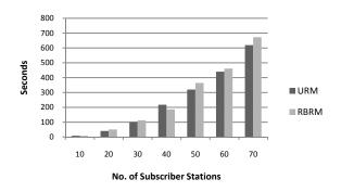
Fig. 10. Total end-to-end delay for nrtPS
