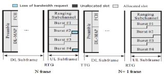
Fig. 2. Recovery of bandwidth requests with RBRM approach
