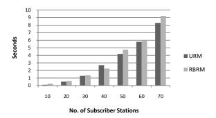
Fig. 11. Total end-to-end jitter for nrtPS
