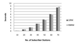
Fig. 17. Total end-to-end jitter for nrtPS in different modulation scheme and coding
