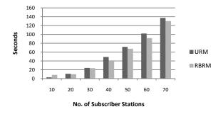
Fig. 8. Total end-to-end jitter for rtPS
