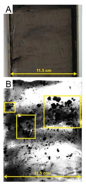
Fig. 2. A representative example, at the macroscale, of a core from Scoresby Sund (PS1718-1): A) Split core half as seen with the naked eye; B) X-radiograph (yellow boxes indicate coarse-grained 'dumps' of material).
