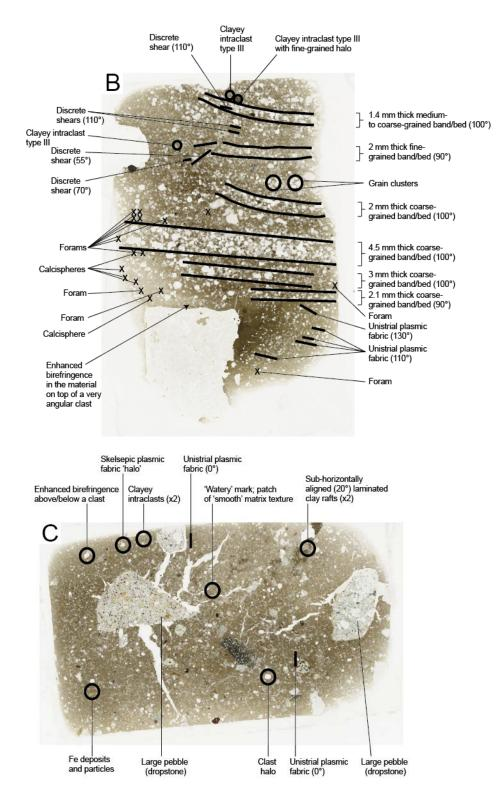
Fig. 4. A representative selection of annotated full thin section scans: A) PS1721-1D, from a zone of high-intensity iceberg scouring (maximum width of sediment in the thin section is 36 mm); B) PS1727-1A, from a zone of intermediate-intensity iceberg scouring (maximum width of sediment in the thin section is 35 mm); C) PS1719-1A, from a zone of low-intensity iceberg scouring (maximum width of sediment in the thin section is 60 mm).
