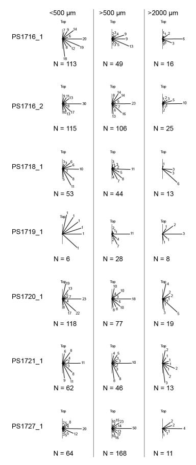
Fig. 6. Clast microfabric for grain size categories <500 μm, >500 μm and >2000 μm in all seven cores. Number of grains measured at specific orientations are indicated on each rose diagram. N = total number of grains measured. Note that the total number of grains measured in each core is the combined thin section data from each core.
