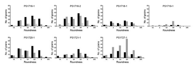
Fig. 5. Clast roundness for grain size categories  $<500 \mu m$  (black),  $>500 \mu m$  (dark grey) and  $>2000 \mu m$  (light grey) in all seven cores. VA = Very Angular; A = Angular; SA = Sub-Angular; SR = Sub-Rounded; R = Rounded; WR = Well-Rounded (after Powers, 1953). Note that the total number of grains measured in each core is the combined thin section data from each core.
