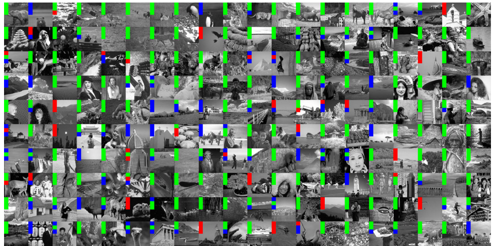
Fig. 11 Ordering of regularisers with batch learning, L_\eta^1 \nabla cost, and noise variance \sigma^2 = 2 , on the 200 images of the BSDS300 dataset, resized. Best regulariser: red TV, green ICTV, blue TGV 2 ; top SSIM, middle PSNR, bottom objective value
