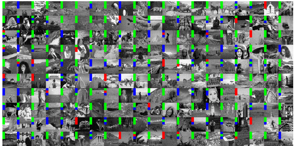
Fig. 13 Ordering of regularisers with batch learning, L_\eta^1 \nabla cost, and noise variance \sigma^2 = 20 , on the 200 images of the BSDS300 dataset, resized. Best regulariser: red TV, green ICTV, blue TGV 2 ; top SSIM, middle PSNR, bottom objective value
