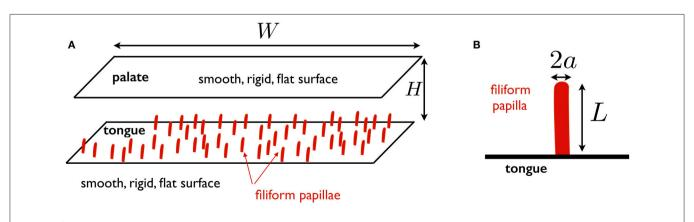
**FIGURE 1 | (A)** Schematic representation of mouth model used in this work. The palate and the tongue are assumed to be smooth, rigid, flat surfaces. The tongue is located at a distance H from the palate and the total width of the fluid region in the anterior-posterior direction is denoted W; **(B)** Schematic representation of papilla model: a straight elastic rod of length L, radius a, clamped on the tongue.
