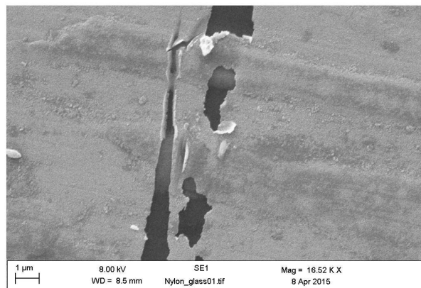
Figure 4: SEM scan of polymer deposit along the sliding track. The obvious vertical scars result from a small scratch on the surface, which seems to have lifted the polymer transfer film away from the underlying glass.
