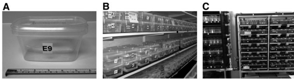
FIG. 1. Static pot system used during the genotyping procedure. (A) Image of one pot. (B) Image showing the scale of implementation at the Wellcome Trust Sanger Institute. (C) Image of the genes rack on system.
