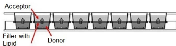
Figure 2.1 – Cross section of the PAMPA Explorer™ sandwich plate sold by BioTek Instruments, Inc. ( www.biotek.com ). The flux of molecules across a filter supporting a lipid bilayer is measured using UV spectroscopy.
