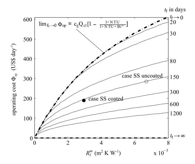
Figure 5: Impact of fouling model parameters  $t_f$  and  $R_f^{\infty}$  on the optimal operating cost for the uncoated SS unit in Table 1. Dash-dot line shows where the criterion  $\chi < 0$  applies. Dashed line indicates the no-fouling case. Case study units: ( $\circ$ ) uncoated SS unit, ( $\bullet$ ) coated SS unit.
