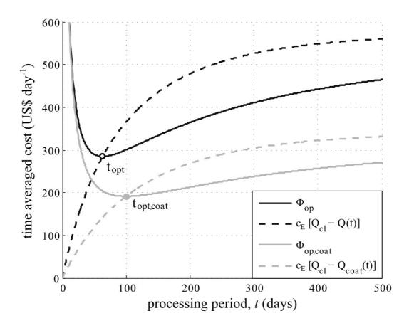
391Figure 4: Effect of processing period length on the annualised operating cost,  $\phi_{op}$ , and the thermal cost392of fouling for the uncoated and coated SS heat exchanger.
