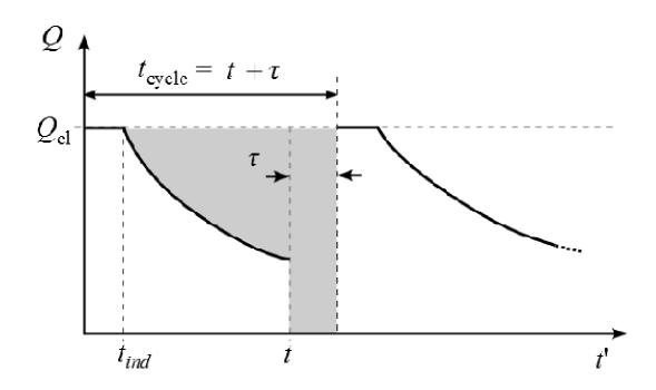
378Figure 1: Schematic of the fouling-cleaning cycle in a single heat exchanger subject to fouling over379time t'. Following an induction period of length  $t_{ind}$ , the duty Q falls from the clean value  $Q_{cl}$ .380After operating for length t the unit is cleaned, taking time  $\tau$ , and performance is restored to381 $Q_{cl}$ . Grey shaded area represents energy lost.
