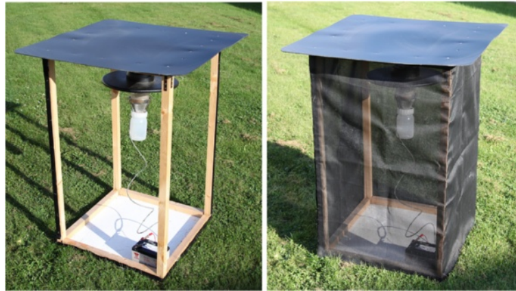
Fig. 3 Field Trial One: Equipment utilised to investigate the effectiveness of insecticide-treated mesh in preventing entry of Culicoides . Ultraviolet (UV) Center for Disease Control (CDC) light-suction trap (model 912: John W Hock, FL, USA) hung within an open-sided wooded frame (width: 1.0 m; length: 1.0 m; height: 1.2 m), with solid black roofs extending 10 cm in each direction, and solid white wooden base. The sides of each frame were either: (i) covered with insecticide-treated mesh, (ii) covered with untreated mesh, or (iii) left uncovered without mesh
