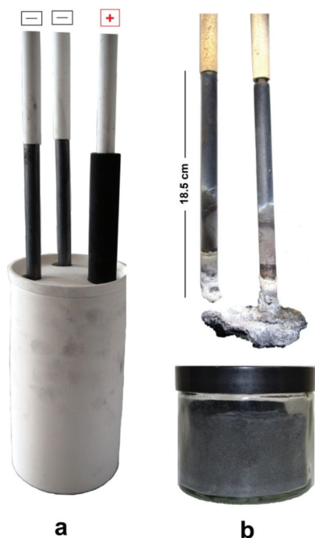
Fig. 5 (a) Photograph of the electrolysis cell. Two graphite rods served as alternative cathodes during the molten salt process. The arrangement of the electrodes in an alumina crucible containing LiCl, before loading into the molten salt reactor can be seen. (b) Photograph of the graphite electrodes after being used as the cathode during the molten salt process. Part of the graphite cathodes exposed to the molten salt (about 11.5 cm) was completely exfoliated into graphene. Distilled water was added to the alumina crucible in order to dissolve the solidified LiCl, resulting in the retrieval of 70 g graphene material, which was stored in a jar after vacuum filtration and drying.
