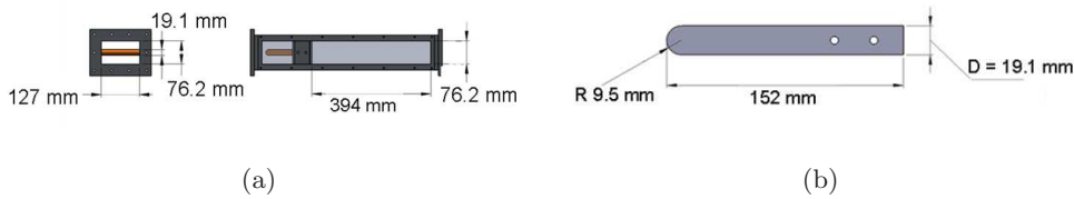
FIGURE 3. Drawings of a) the test section and b) the bluff body
