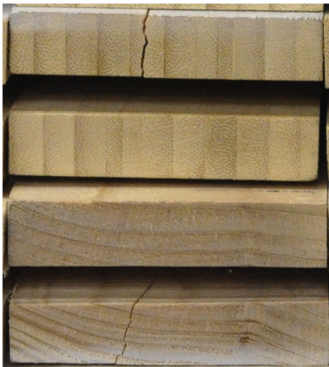
Fig. 7. Cracks in bleached bamboo (top) and Sitka spruce timber (bottom) – the crack in the bleached bamboo is typical in orientation for all bamboo specimens.
