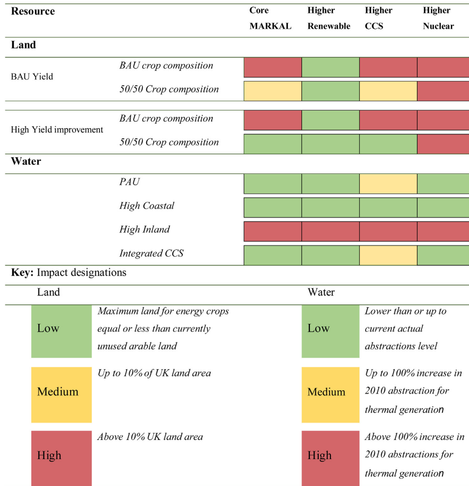
Fig. 5. Environmental no-regrets matrix. The categories of impacts on land and water presented here are independently assessed based on different metrics of identifiable limits of sustainable land appropriation and water use.
