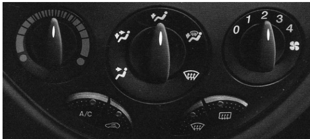
Figure 3: Heating controls for the 1999 Ford Focus, where the centre knob for distribution control is larger than the knobs either side of it. Image source: Malcolm (1998).
