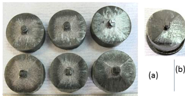
Figure 1. (a) Six GdBCO–Ag single grains grown using buffers, employing top seeded melt growth process and (b) one YBCO single grain of diameter 25 mm grown using the buffer-aided infiltration growth technique.
