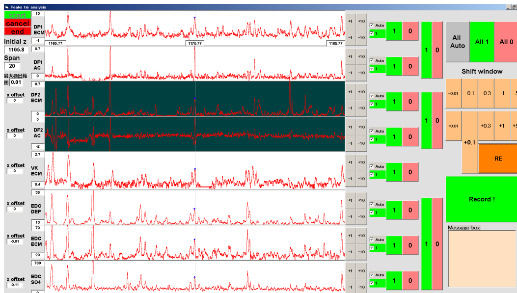
Figure 2. A PC interface window used to search for tie points semiautomatically. Based on preliminary tie points, a detailed search can be conducted easily. In the data profiles (red traces), the candidates for tie points were found by extracting local maxima (dots in the center of graphs). After choosing each datum or not (1/0 switches in the right side of the image), by clicking “Record” on the right, the data – depth of peak, peak height and background level – are recorded. This example is for a plausible Toba super eruption that occurred sometime at \sim 74 ka studied by Svensson et al. (2012). Graphs from the top are: DF1 ECM, DF1 ACECM, DF2 ECM, DF2 ACECM, Vostok ECM, EDC DEP, EDC ECM and EDC sulfate (see Table 1).
