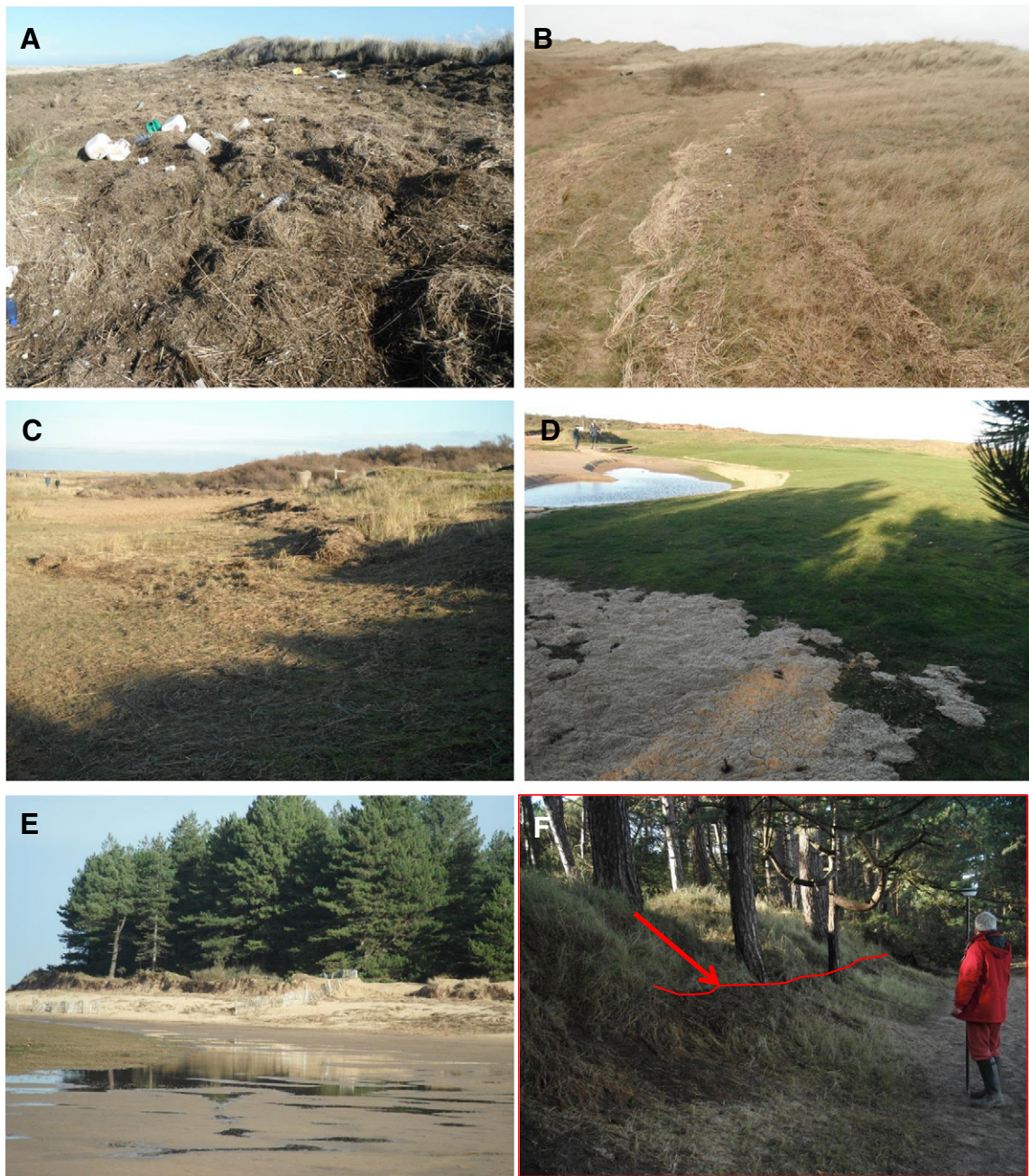
Fig. 8. Local variations in surge water levels, North Norfolk coast. A) Massive debris bank reaching 5.95 m ODN, Privet Hill, Scolt Head Island; B) typical back-barrier driftline (furthest right in image) at 5.52 m ODN, Great Aster Marsh, Scolt Head Island; C) drift at up to 6.30 m ODN on exposed seaward-facing dunes, Holme; D) water level line at limit of storm surge inundation (4.43 m ODN), Holme Golf Course; E) cliffling on seaward margin of Holkham Gap embayment (peak level of drift in dunes = 6.37 m ODN); F) driftline in pine plantation, Holkham Gap (water level 500 m to west = 4.46 m ODN).
